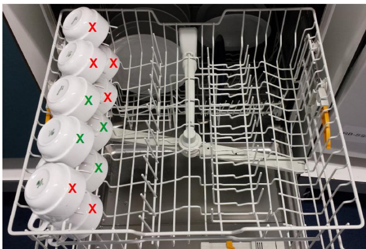
Figure 19: Photograph of the placement of the tea cups being assessed for bleaching in the dishwasher test. X = Cups which are evaluated for bleaching performance, X = Clean cups which remain in the dishwasher to ensure even heating
