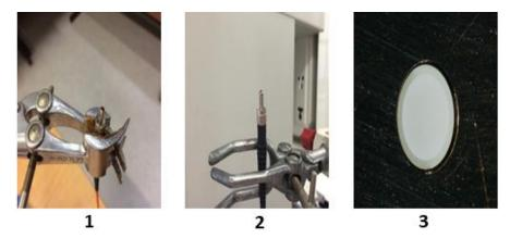
Figure 4-2: Polishing steps for the SMA905 Fibre connectors.1-Hang the connector in a safe spot after inserting fibre into epoxied connector.2- Protrude fibre to make ready for polishing. 3- Fibre after polishing.
