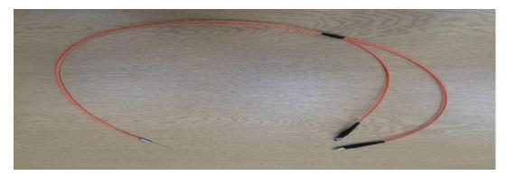
Figure 4-4: The physical optical probe
