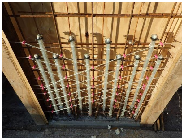
Figure 5.12: Layout of SMP tendons and flow networks in panel B.
