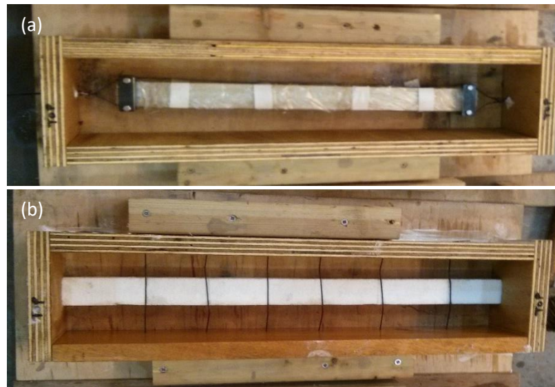
Figure 4.6: (a) PET beam sample set-up (white tape was removed before casting); (b) PETr beam sample set-up (with polystyrene void-former).
