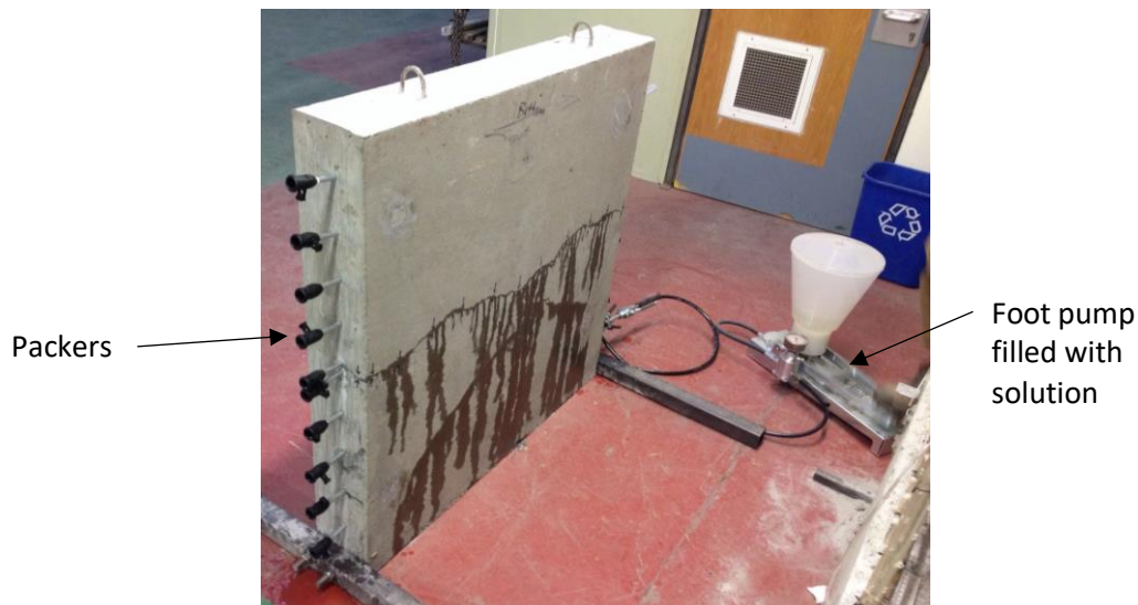
Figure 5.31: Flow network pump and packer arrangement during laboratory testing.
