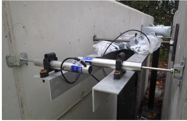
Figure 5.29: LVDTs 2-5, positioned to measure displacements of the trial panel and reaction wall.
