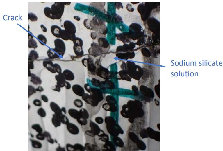
Figure 5.45: Sodium silicate solution exiting from the crack during pumping of flow networks.
