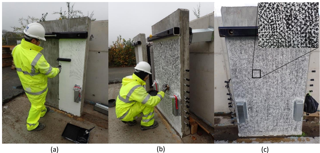
Figure 5.27: Application of DIC speckle pattern to trial panels (a) uniform spots; (b) uneven application using wooden block; (c) final pattern.
