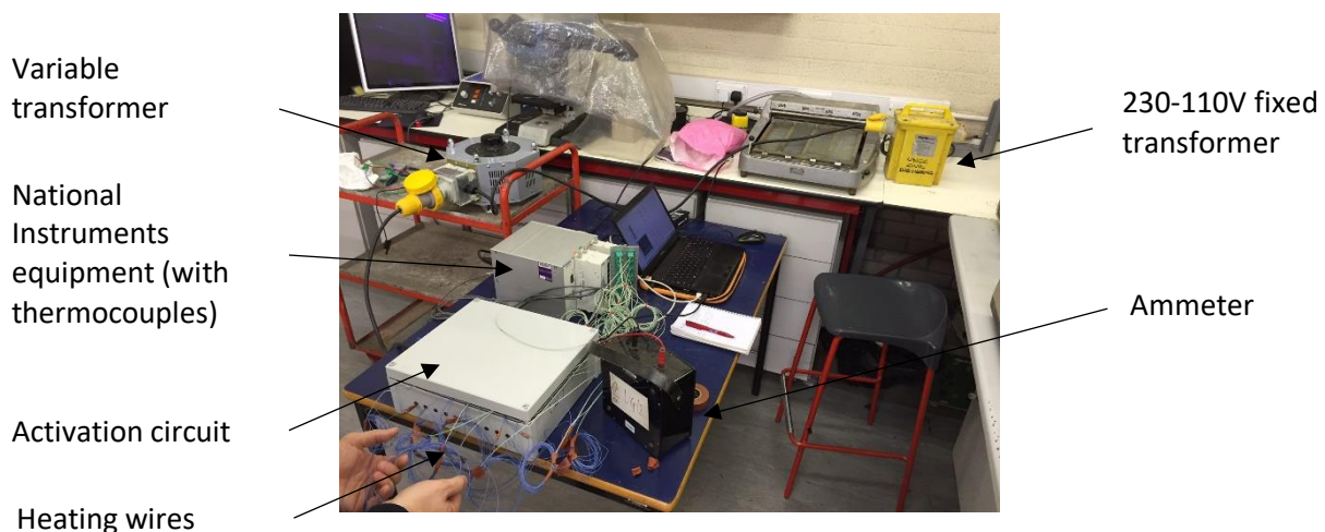
Figure 5.25: Activation system lab test setup.
