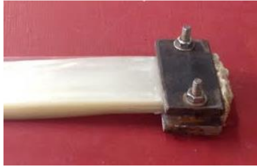
Figure 4.2: PET strip anchorage arrangement.
