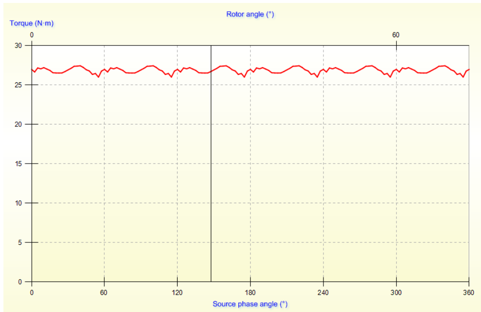
Figure 4.14 FEA analysis of Electromagnetic generated torque of the benchmark design
