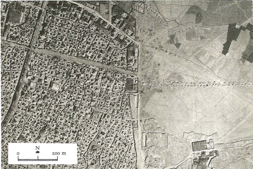
Fig. 3.16: Several qanats in Kirman seen as series of shafts stretching from mother well to the city (source: Kheirabadi 1991)
