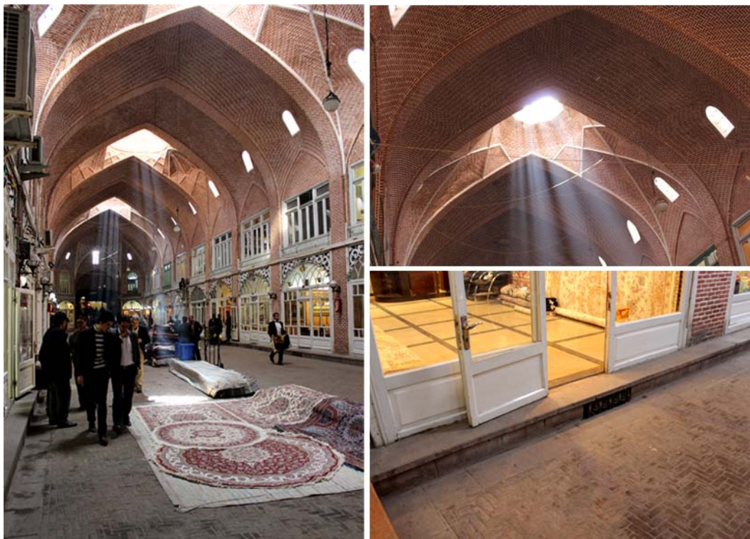
Fig. 2.28: Brick is the main material used in Mozaffarieh Bazaar in Tabriz to form paving, walls and roof structure (source: Author 2013)
