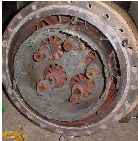
Figure 2.2: Photograph of damaged GT combustion chamber due to excessive combustion dynamics. Reproduced from [16].
