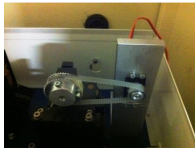
Figure B.18: Schematic of scanning laser sheet PLIF measurement system timing and image capture setup at Cardiff University's GTRC (top) and photograph of servo installation in the TDL-90 dye laser (bottom).
