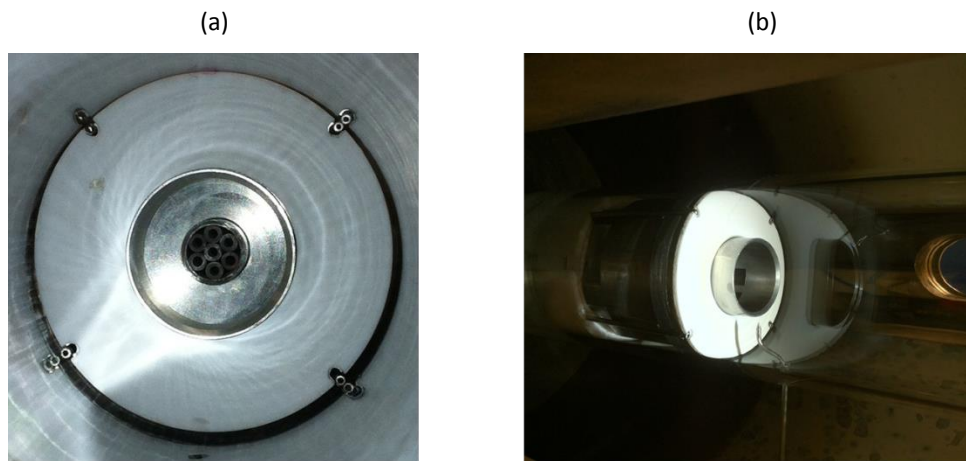
Figure B.10: Photographs of HPGSB-2 burner components with an end-on view of the burner face, exit nozzle, and instrumentation/pilot lance prior to installation in the HPOC (a) and after installation in the HPOC with the spark igniter installed (b).
