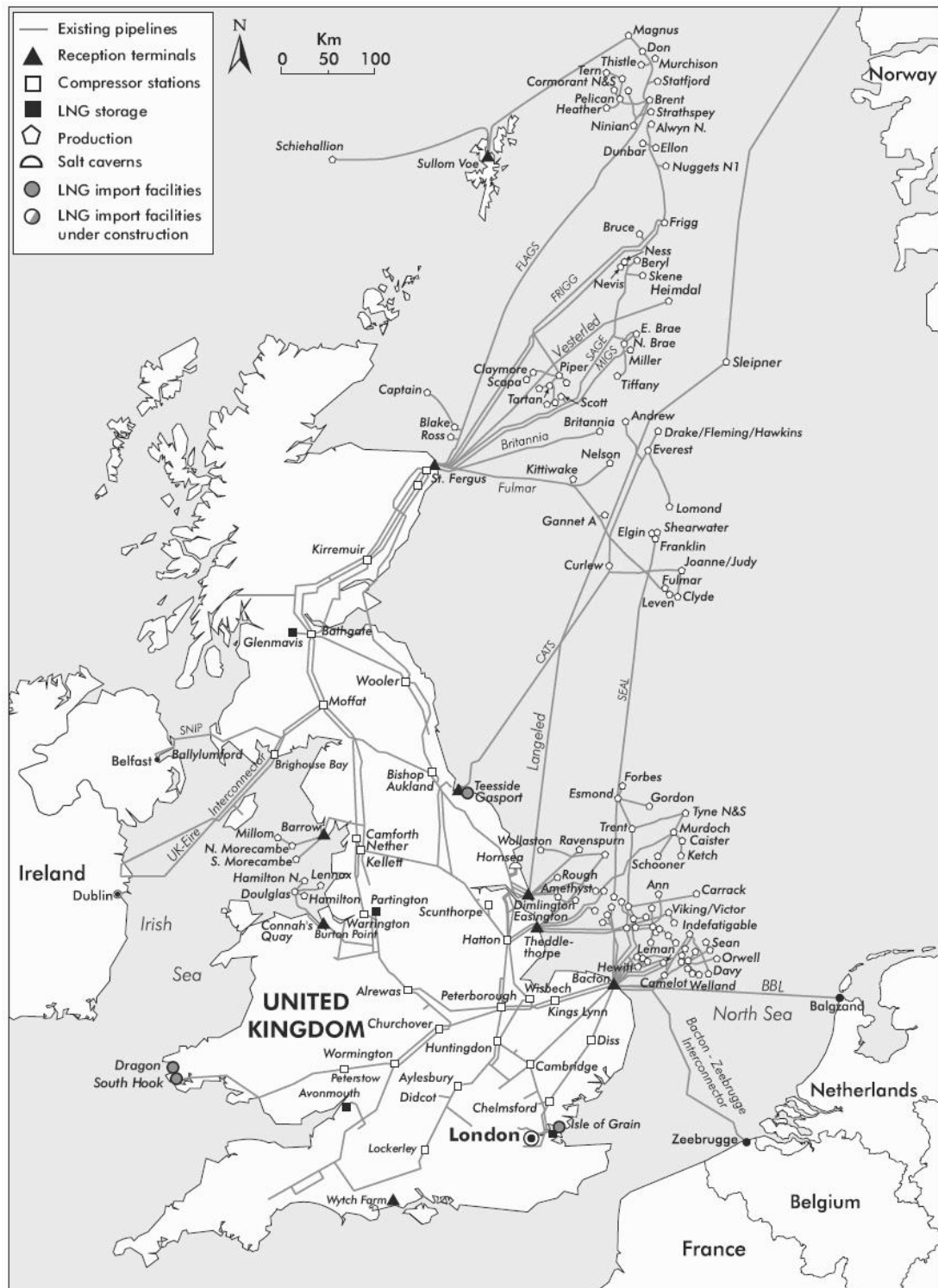
Figure A. 1: UK gas transmission network including LNG import facilities and interconnectors. Reproduced from [19].
