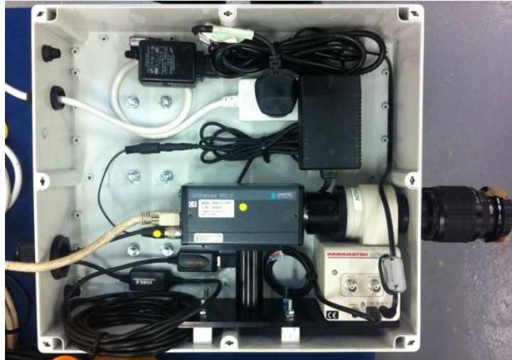
Figure B.12: Photograph of the ICCD camera system as installed in the IP-67 enclosure. Refer to Figure 3.2 for installed location in the HPCR.
