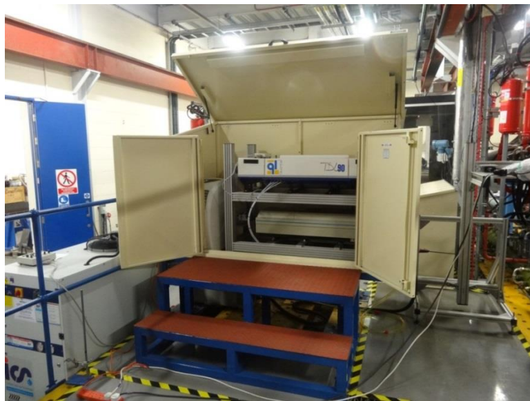
Figure B.13: Photograph of PLIF laser system as installed at Cardiff University's GTRC.
