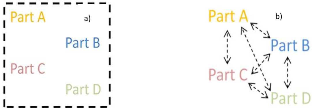
Figure 2-1 contact domain a) general contact; b) contact pairs, (Abaqus 2013)
