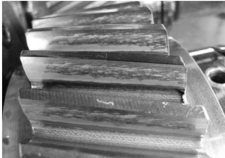
Figure 1-19 Micropitting predominantly in the dedendum region of a helical test gear tooth ( Evans et al. 2013).
