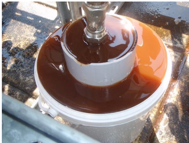
Figure 7.5 Red colour showing washout of media during hydraulic conductivity test at University
