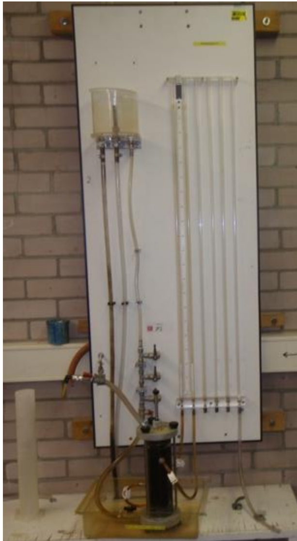
Figure 3.15 Laboratory constant head hydraulic conductivity test
