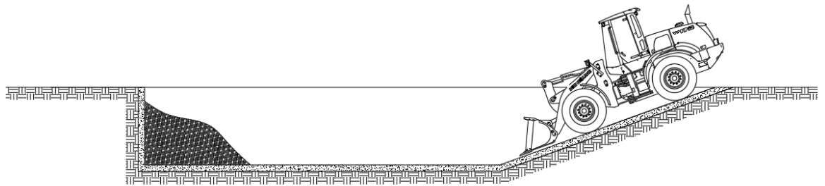
Figure 9.13 Front slope in system and concrete base to allow replacement of media
