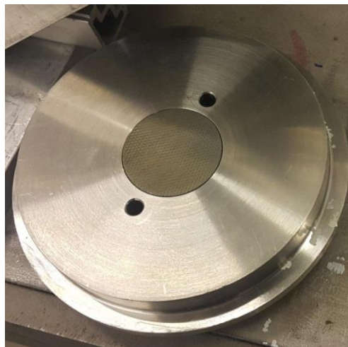
Figure 5-10 manufactured surface insert and the large disc.
