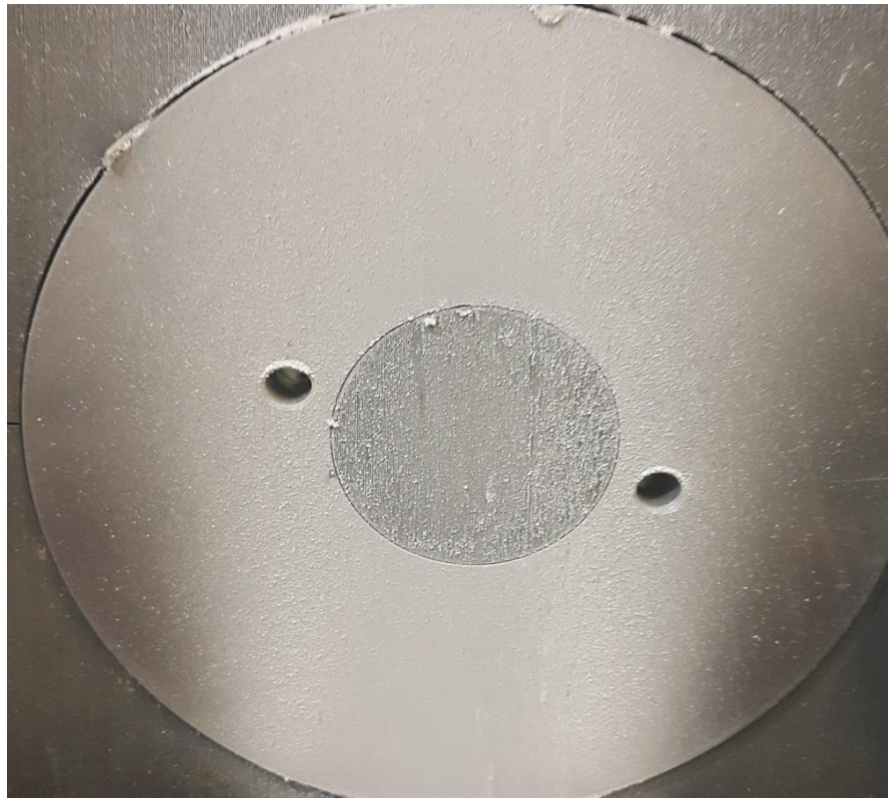
Figure 7-5 seeding deposit on riblet surface (scallop surface).
