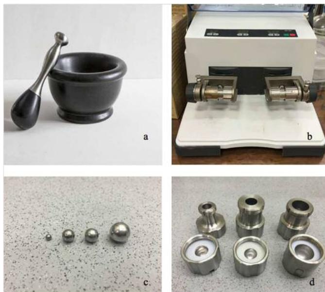
**Figure 1.** (a) pestle and mortar; (b) The Retsch MM-400 mixer mill; (c) stainless steel balls; (d) stainless steel jars
