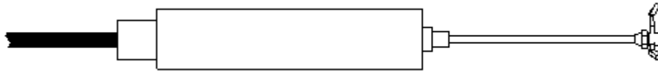
(a) - Parts of a velocimeter probe. From left to right: cable, conditioning module, measuring probe
