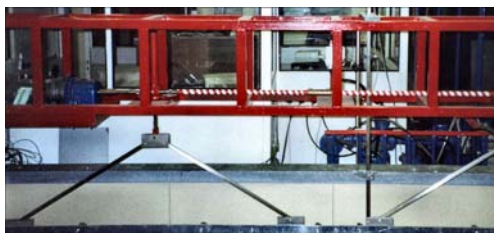
(c) Weir gate drive mechanism
