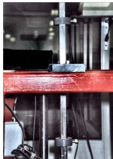
(e) Safety switches
