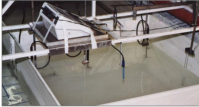
(a) - Three ADVs, wave probe monitor and conductivity meter in operation
