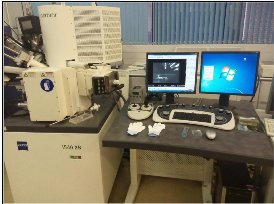
Figure 4.6: The SEM instrument utilised
