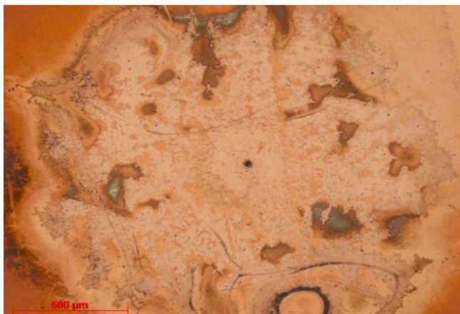
Figure 19. Polished copper plane electrode after 1 lightning impulse breakdown to the surface as observed through an imaging microscope (bright light setting).
