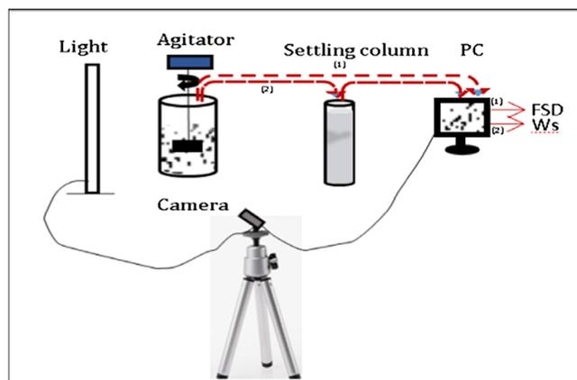
**Fig. 2** Schematic diagram of the PIV system, settling column, sample bowl and stirrer
