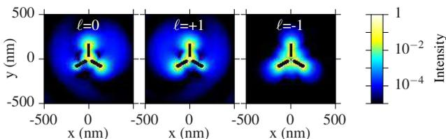
Figure 4: Electric field calculated with the BEM. The intensity in the  $z = 0$  plane is shown on a logarithmic scale for  $\ell = 0, +1, -1$  from left to right. A movie of the time behavior of the fields can be found in the supplementary information.
