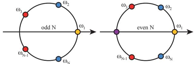
Figure 5: Sketch of the possible resonance frequencies and their degeneracy for an odd (left) and even (right) number of arms. Same colors imply that the modes are degenerate.
