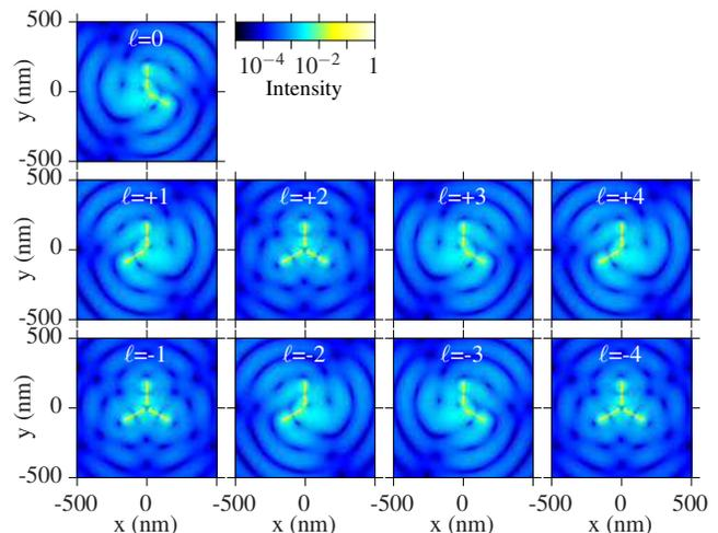
Figure 3: Induced electric field calculated with the antenna model. The intensity in the  $z = 0$  plane with a logarithmic scale is shown for  $\ell = 0$  (top) and positive OAM  $\ell = 1 \dots 4$  (middle) and negative OAM  $\ell = -1 \dots -4$  (bottom). A movie of the time behavior of the intensity for  $\ell = 0$  and  $\ell = \pm 1$  can be found in the supplementary information.
