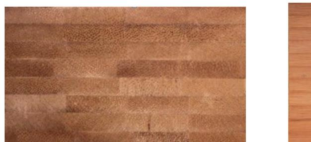
Figure 1.4 (a): Laminated bamboo panel front view (b): section view
