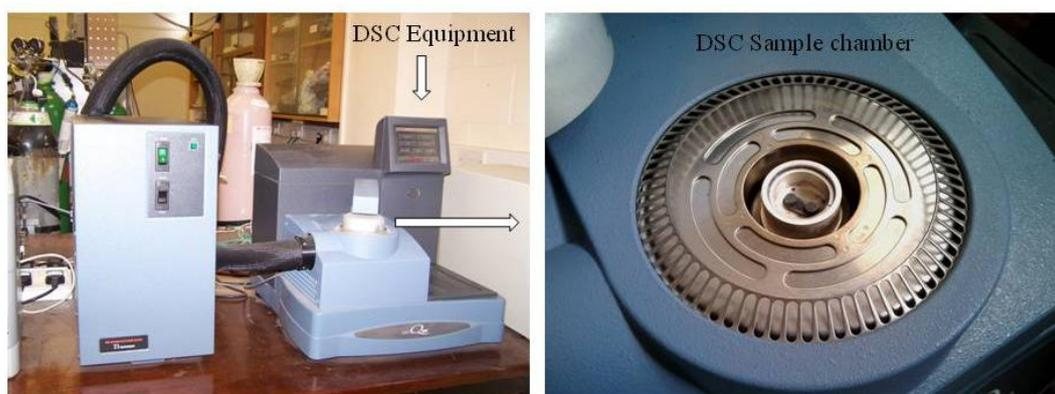
Figure 2.2 Differential scanning calorimeter (DSC)
