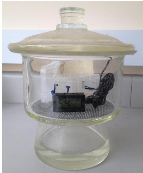
Figure 8.2.2 The desiccator assemblies for the hygroexpansion experiment
