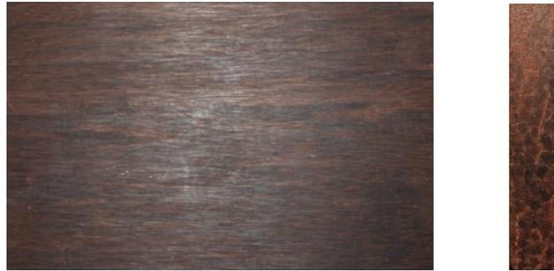
Figure 1.1 (a): Recombination bamboo panel front view (b): section view
