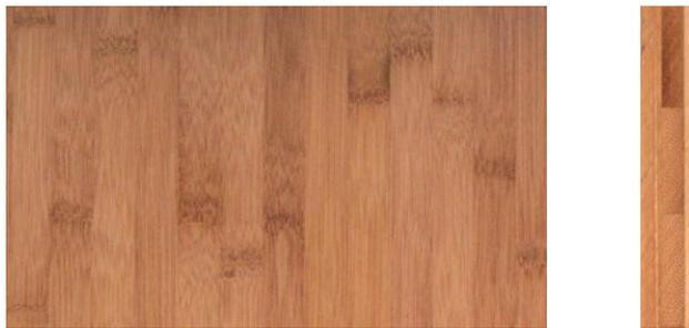
Figure 1.6 (a): Laminated bamboo panel front view (b): section view
