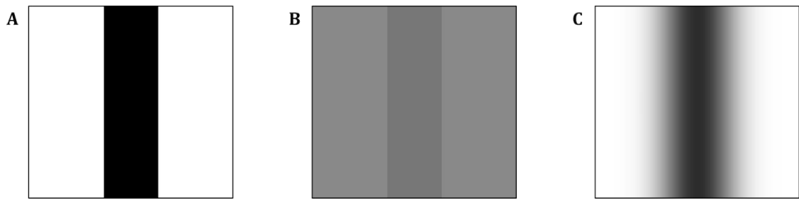
Figure 2.16 Schematics demonstrating both criteria: (A) optimum image quality, Grade 5; (B) low contrast; (C) low edge definition.
