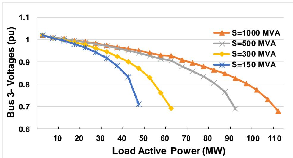
Figure 3- 6: P-V curves of the AC grid without an energy source for different short-circuit levels
