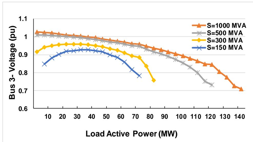
Figure 3- 7: P-V curves of the AC grid with an energy source for different short-circuit levels
