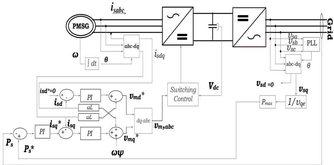
Figure 2- 2: Full power converter control block diagram [112]
