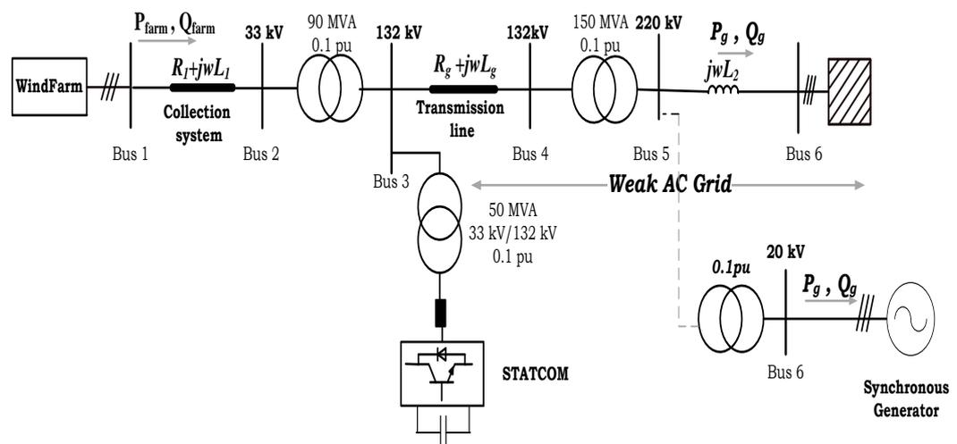
Figure 4- 17: Dynamic Model of Test System
