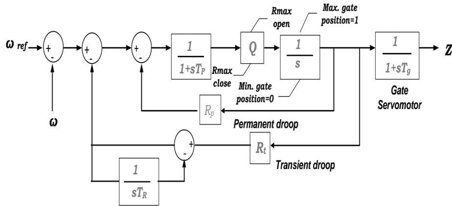
Figure C- 2: Mechanical –Hydraulic Control (GOV1)
