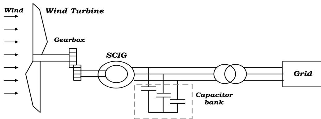
Figure 1- 2: Fixed-speed wind turbine with a SCIG
