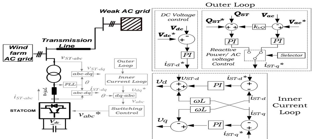
Figure 4- 8: Control structure of the STATCOM
