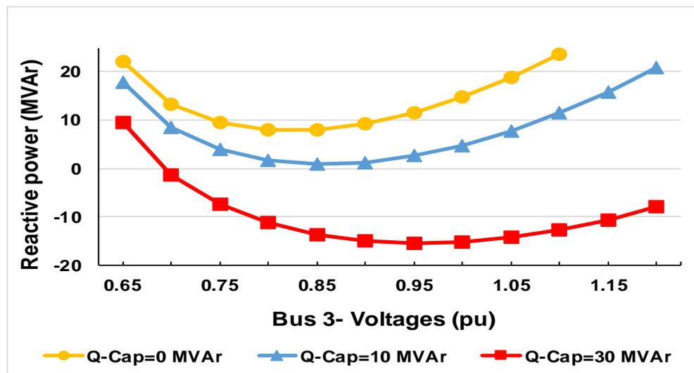
Figure 3- 11: V-Q Curves of weak AC grids
