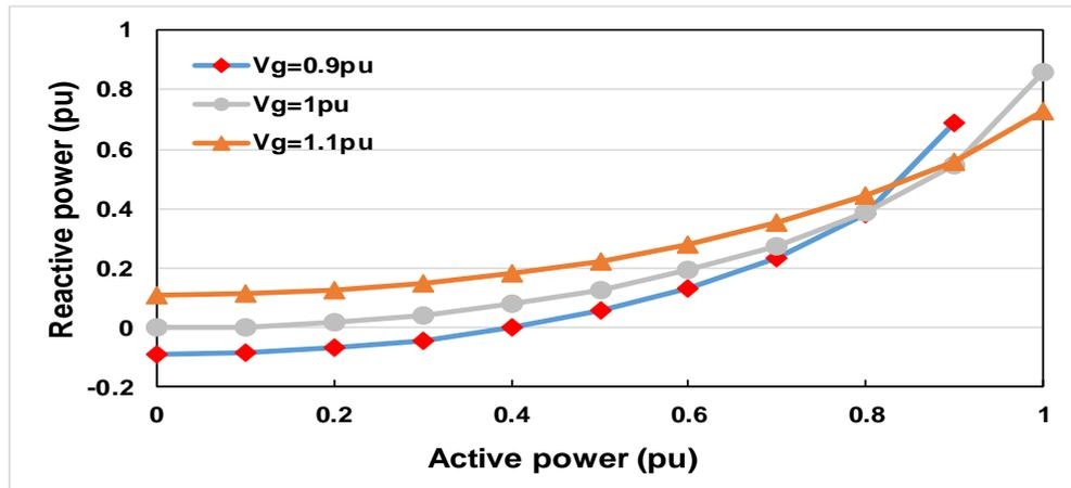
Figure 4- 4: The PQ curve for different grid voltages
