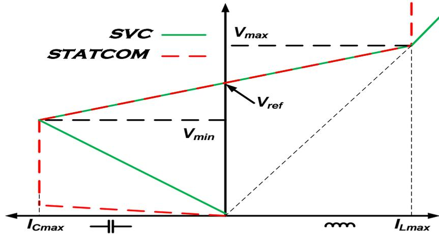
Figure 4- 5: I-V Characteristic of SVC and STATCOM
