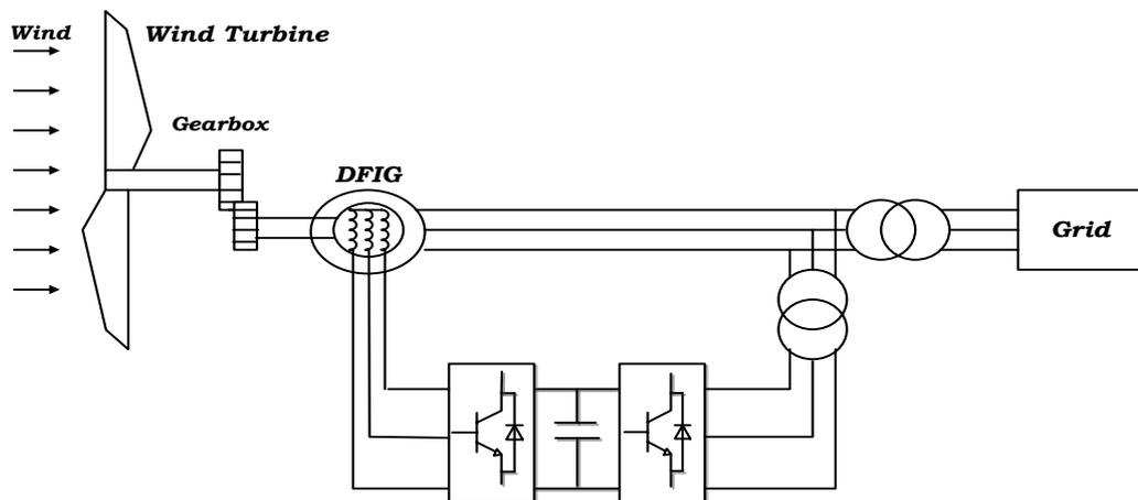
Figure 1- 3: Variable-speed wind turbine with a DFSG
