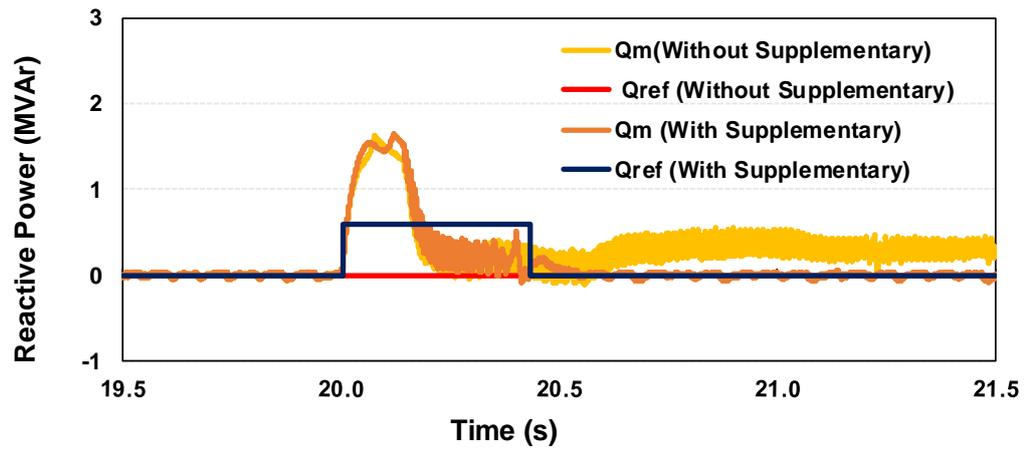
(b) Reference and measured the reactive power of grid side converter
