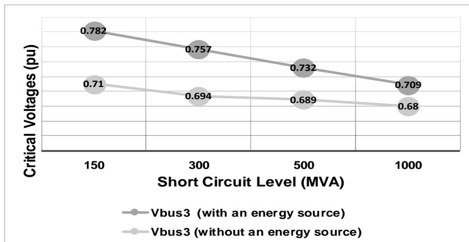
Figure 3- 9: Comparison of critical grid voltages with and without an energy source
