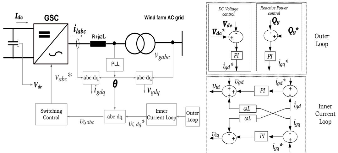
Figure 4- 7: Grid Side Converter Control Scheme
