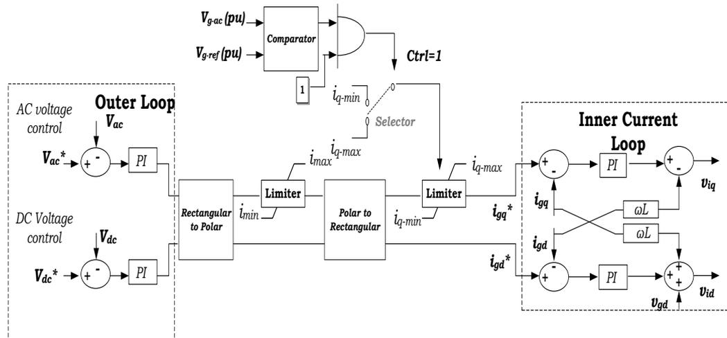
Figure 5- 6: A supplementary control in AC voltage control mode
