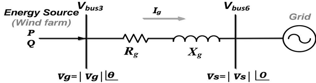
Figure A- 2: The equivalent diagram of the system between bus bars 3 and 6
