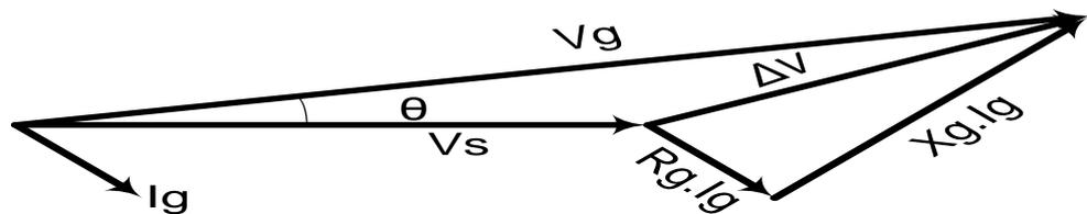
Figure A- 3: The phasor diagram of equivalent system between two bus bars
