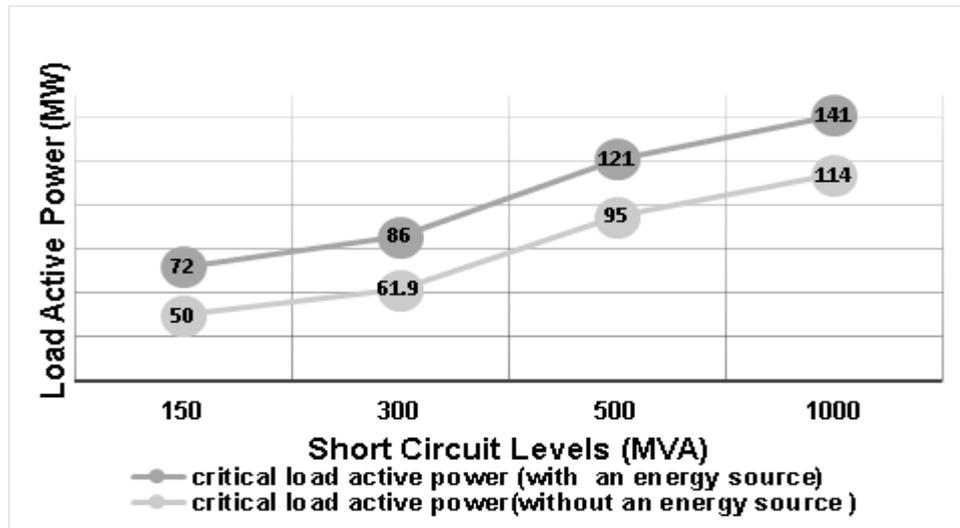
Figure 3- 8: Comparison of critical load active power with and without an energy source
