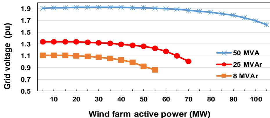
Figure 4- 14: Simulation results of the weak AC grid with fixed capacitors
