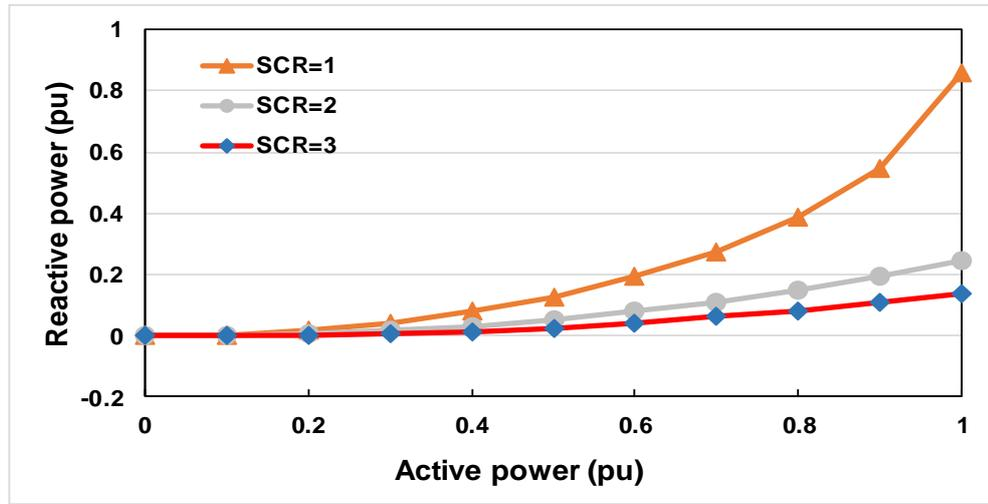
Figure 4- 3: The PQ curve for different SCR values
