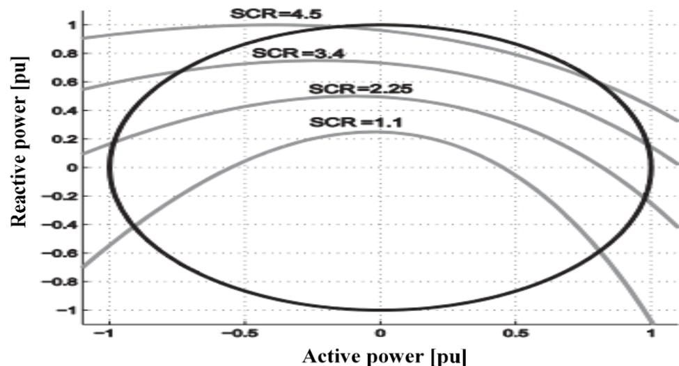
Figure 2- 1: PQ chart for different SCR values at AC grid voltage of 1pu [55]
