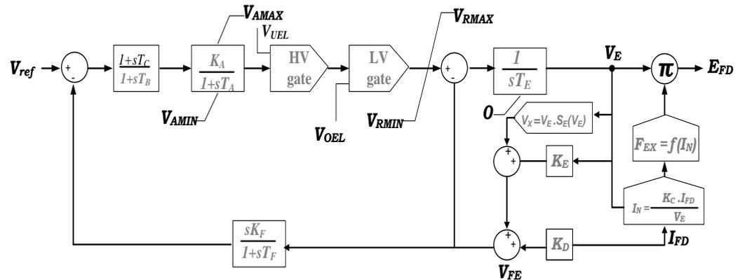
Figure C- 4: IEEE Alternator Supplied Rectifier Excitation System
