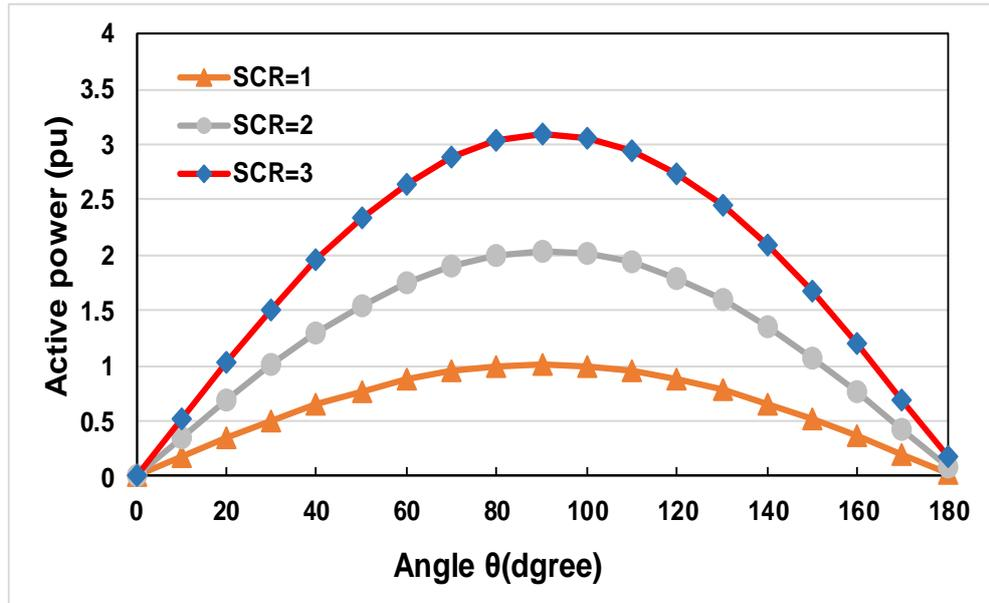
Figure 4- 2: Transferred active power for different grid reactance values
