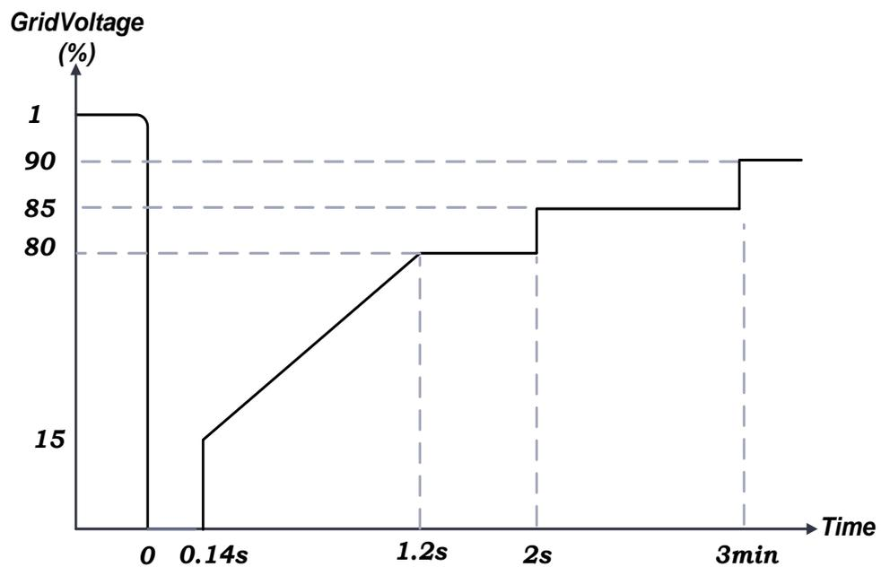
Figure 5- 1: Fault ride-through capability required in GB
