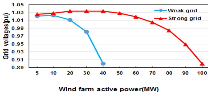
(a) P-V curves for the weak AC grid & the strong AC grid
