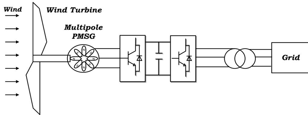
Figure 1- 4: Variable-speed wind turbine with a PMSG
