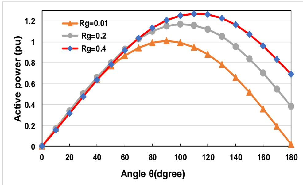
Figure 4- 1: Transferred active power for different grid resistance values
