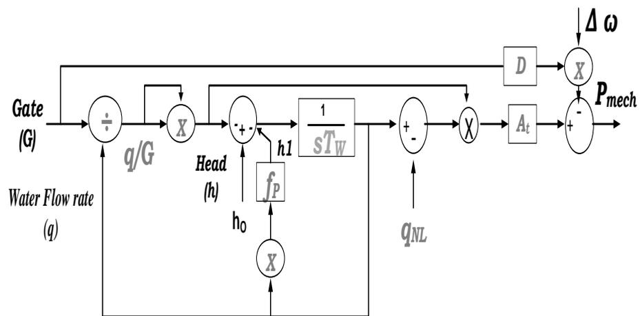
Figure C- 3: Non –Elastic Water Column without Surge Tank (TUR1)
