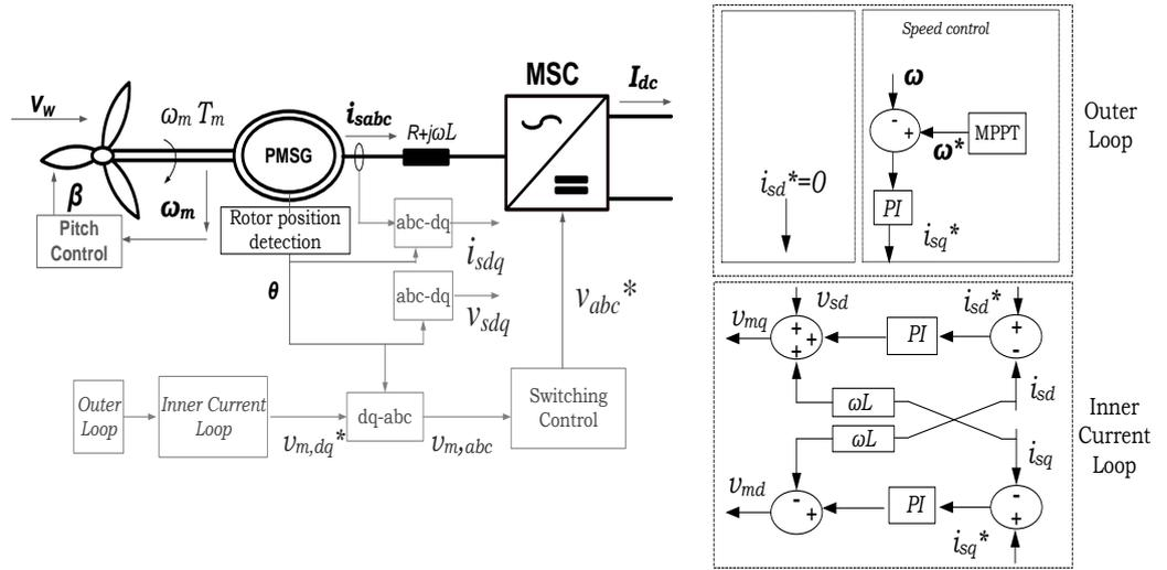
Figure 4- 6: Wind Turbine Side Converter Control Scheme
