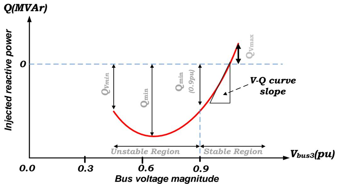
Figure 3- 4: Typical V-Q Curve
