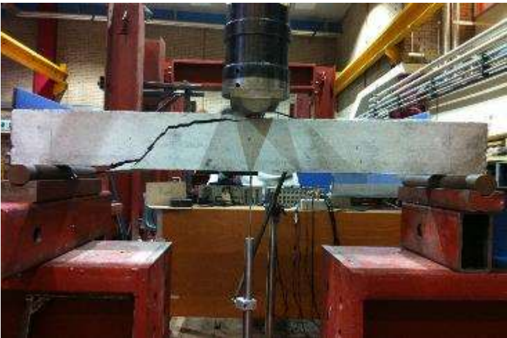
Figure 7.3 Failure mode of the control RC beam
