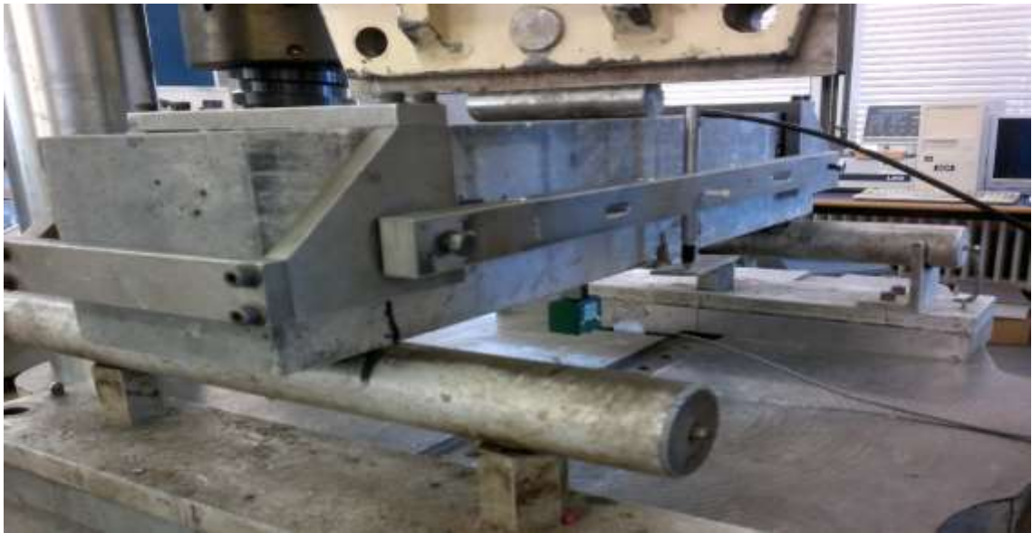
Figure 5.7 Three-point testing configuration.
