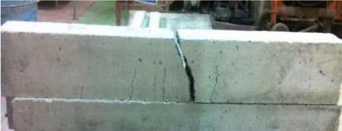
Figure 7.6 Beam sustained 596136 cycles and failed due to rebar fatigue
