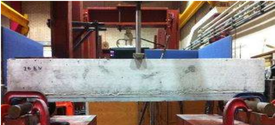
Figure 7.15 Beam sustained 1000000 cycles without any noticeable cracks (maximum cyclic load level 46.91%)
