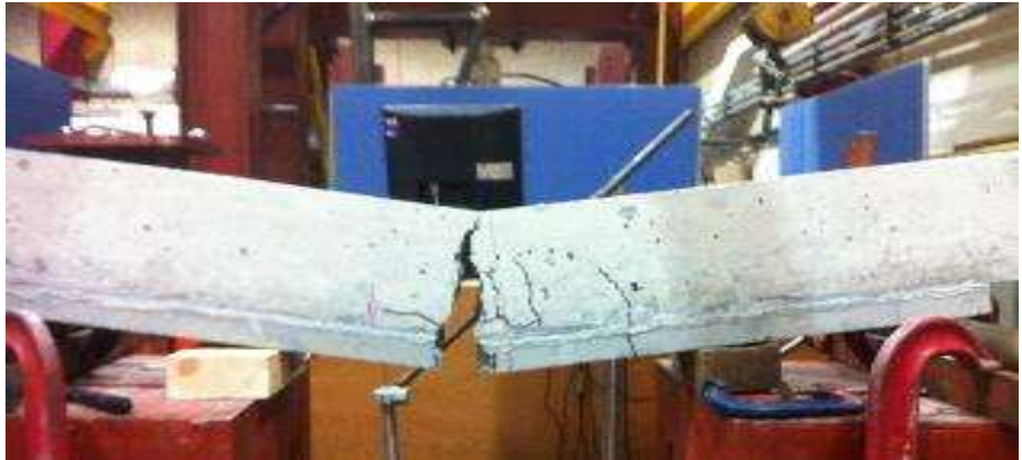
Figure 7.17 Beam sustained 32100 cycles and failed by rebar fatigue (maximum cyclic load level 82.1%)
