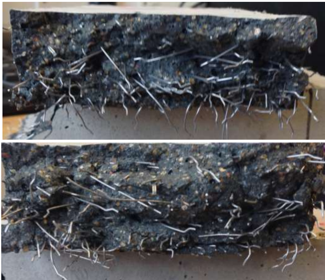
Figure 6.14 Good distribution of fibres in the failure sections
