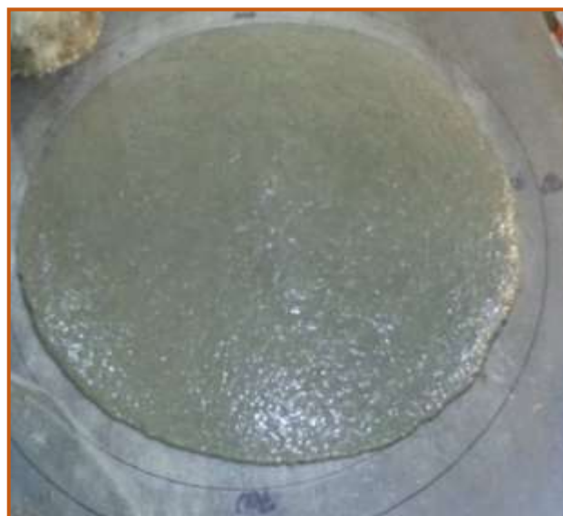
Figure 5.1 Slump flow spread of UHPFRC based on CARDIFRC Mix II
