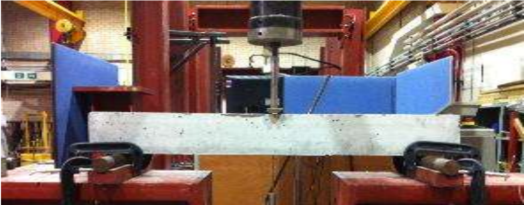
Figure 7.4 Beam sustained 1000000 cycles without any noticeable cracks
