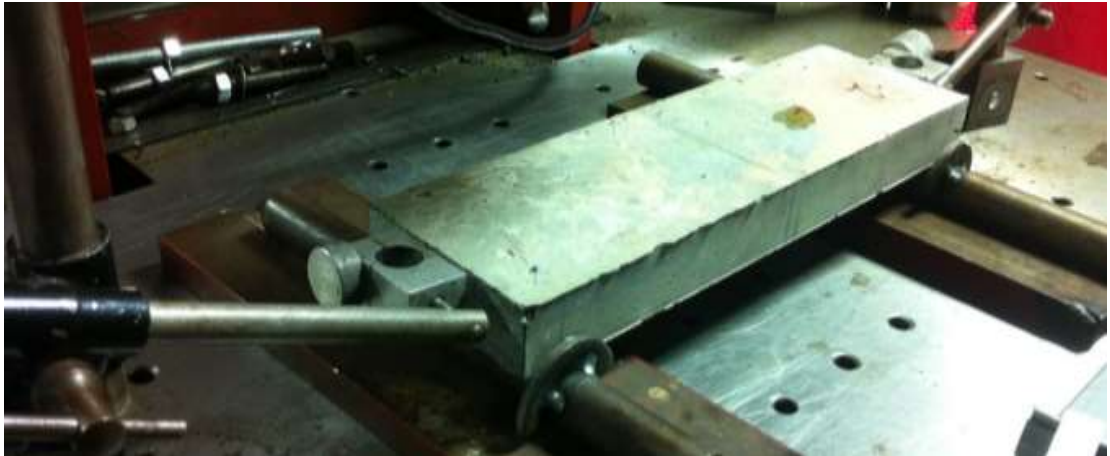
Figure 6.3 Photo of test set up, showing the specimen on simple supports and two mechanical stops. There are two more mechanical stops on the other side of the specimen
