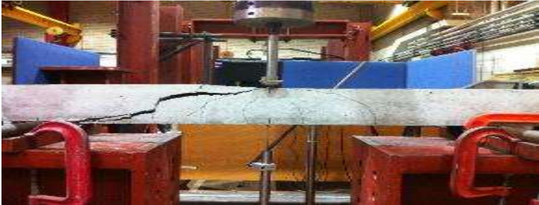
Figure 7.7 Flexural shear crack, beam sustained 11458 cycles
