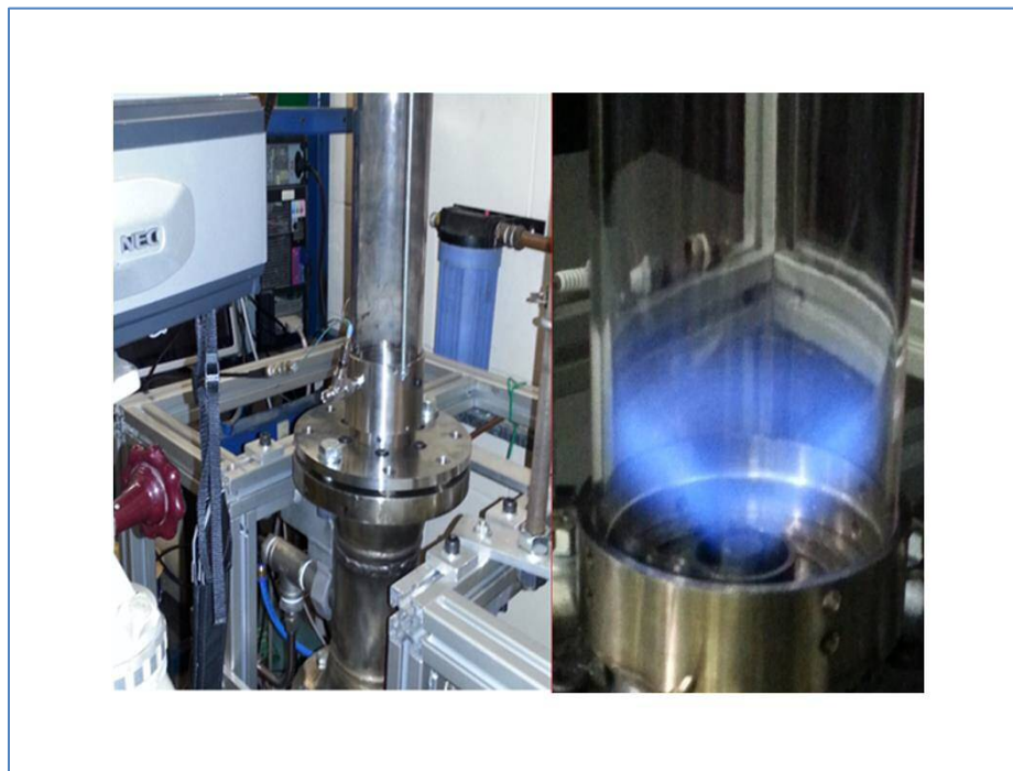
Figure 3. 4 A setup of the swirl premixed burner
