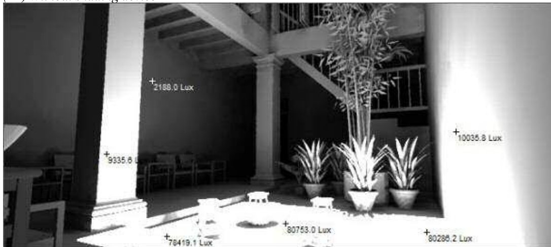
Figure 9.36 (A2 and B2): Selected Radiance renderings (false colour and grey tone) of Courtyard-P2 with adequate sunlight.
