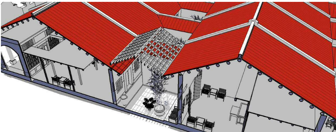
Figure 9.27: The prototype model of solar shading device were proposed at top of front courtyards of the three shophouse case buildings: (a) Courtyard-S 3 ; (b) Courtyard-P 2 ; and (c) Courtyard-D 1 . (Source: Illustration by author, 2015)
