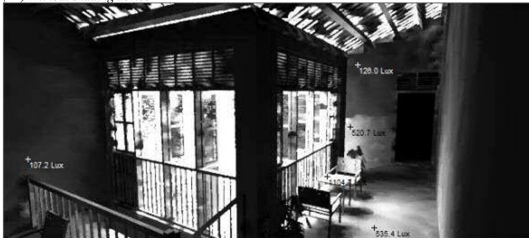
Figure 9.36 (A1 and B1): Selected Radiance renderings (false colour and grey tone) of Courtyard-P2 with adequate sunlight.
