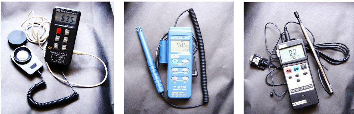
Figure 4.15: The three hand held digital meters for field tests: Datalogging Light Meter by TES-1336A (left); Humidity Temperature Meter by Center-314 (middle); and Hot Wire Anemometer by AM-4204 (right). (Source: Supported and provided by the D.A.U.P., Chung Hua University)
