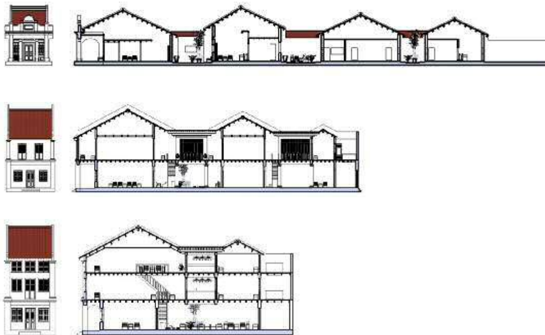
Figure 6.3: Front elevations and longitude sections of the multiple case studies from: single-storey shophouse at Daxi Township in Taiwan (top); double-storey shophouse at George Town in Penang (middle); three-storey shophouse at Chinatown in Singapore (bottom). (Source: Illustration by author, 2008-09)
