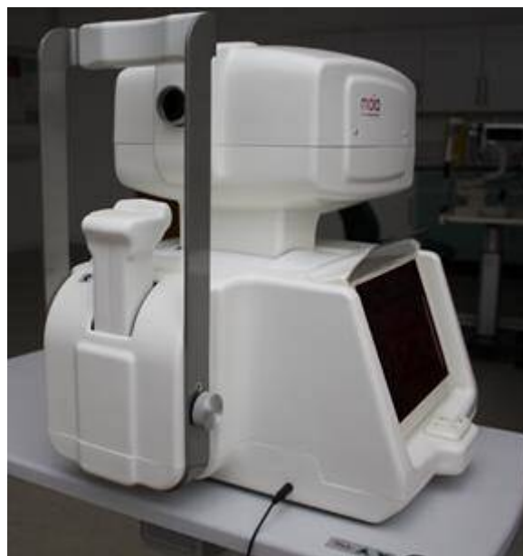
Figure 1.9 The MAIA microperimeter with customised red filter placed on to the computerised screen (right) to avoid excessive light under dark adapted conditions.
