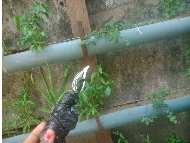
Plate 7-1; data logger wrapped in black cling film
