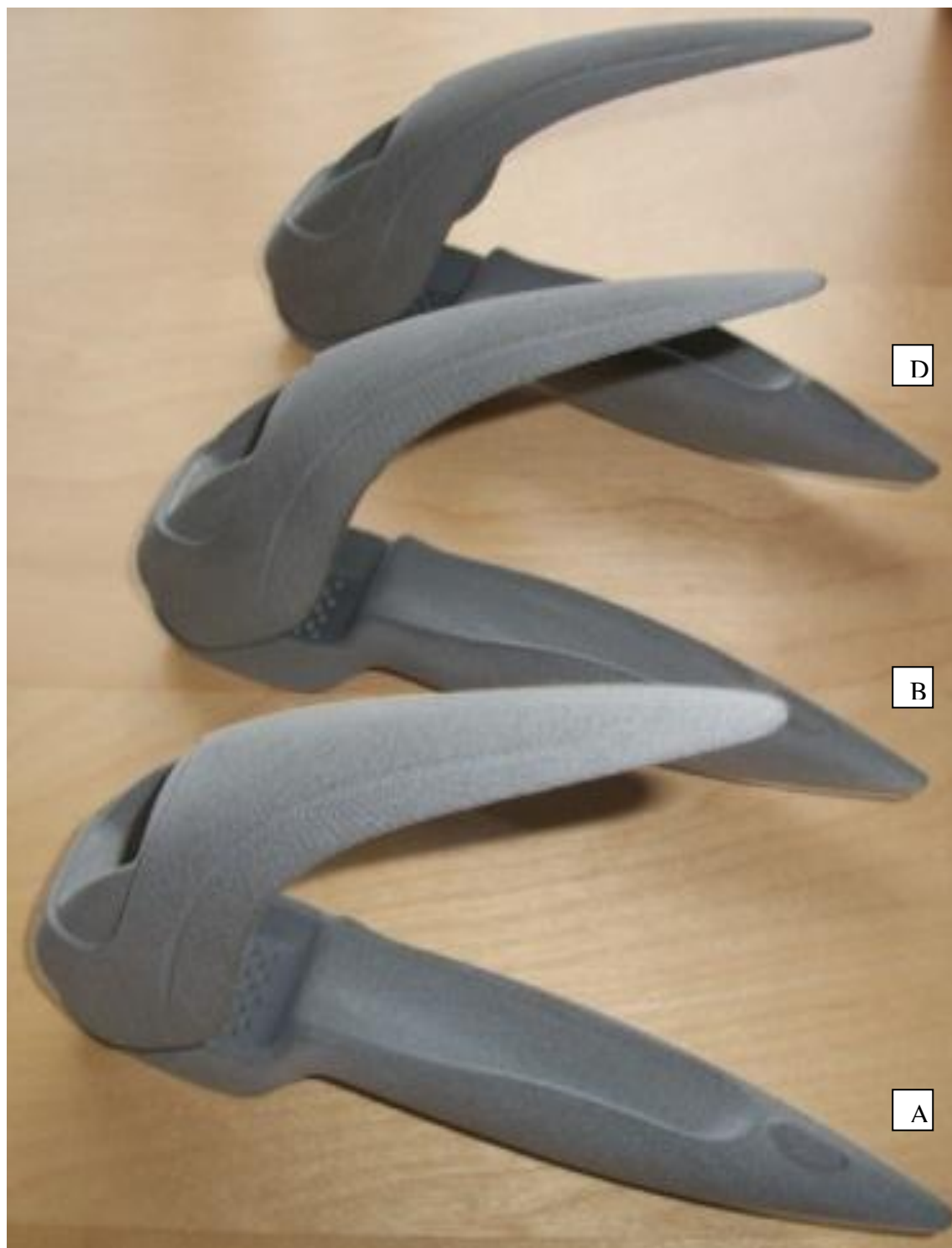
Figure D 1: Illustration of a garlic crusher made of composite material of cement filler with Polyamide 12 (A): 30% cement filler (B) 35% cement filler (D) 40% cement filler.
