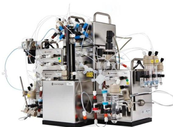
Tracers like  $[^{18}\text{F}]\text{FDG}$ , which require a nucleophilic fluorination followed by a single deprotection step, can be synthesised by these automation modules. Other automation modules like Fastlab from GE healthcare and Trasis (Figure 1.5) allow also more complex synthesis with better radiochemical yields (RCY) and radiochemical purity.
