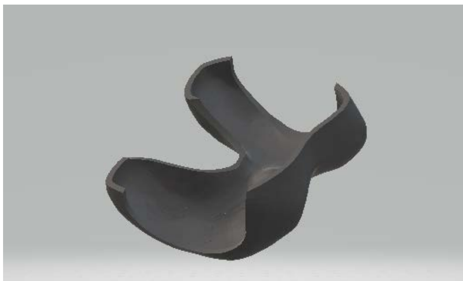
Figure 7.3 Design of 3D printed CoCrMo component
