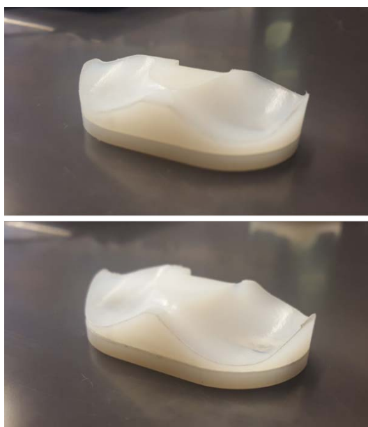
Figure 7.6 Fabricated UHMWPE inserts with amorphous ribbon embedded (Top: insert 1, bottom: insert 2)
