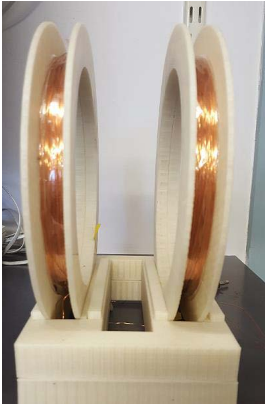
Figure 7.1 Fabricated Helmholtz coils
