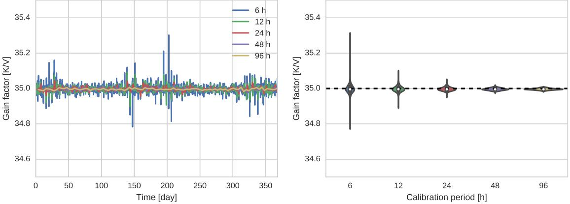
**Figure 21.** *Left:* Variation of the gains estimated in the case of a CMB-only sky. The gain  $G$  used in Eq. (8.9) to produce the simulated timelines was 35.0 K/V. *Right:* Violin plots of the gain estimates shown on the left. Increasing the length of a calibration period reduces the dispersion of the gain estimates.
