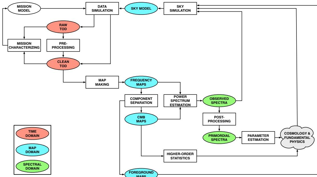
**Figure 1.** A schematic CMB simulation and analysis pipeline, with rectangular operators acting on oval data objects, which may be time samples (red), map pixels (blue) or spectral multipoles (green). Note the many loops, implying iterative processing.
