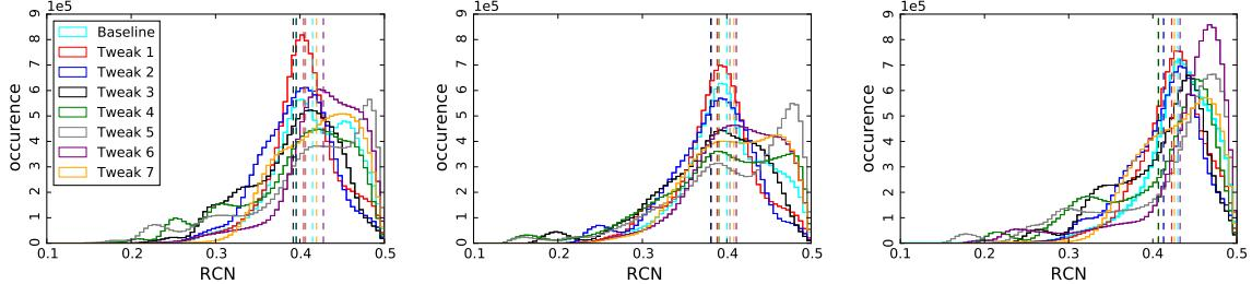
**Figure 7.** Histograms of the RCN for the boresight (left), high (centre) and low (right) detectors in the tweaked cases compared to the baseline (cyan). The vertical dotted lines show the mean values.
