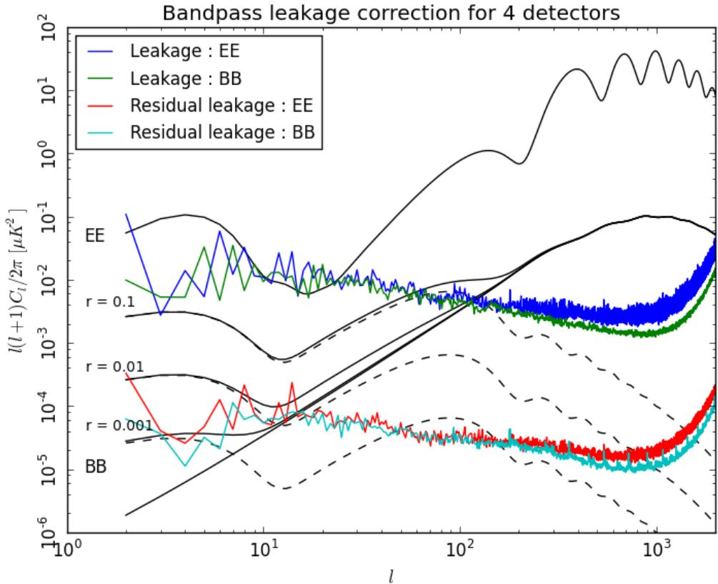
**Figure 13.** *EE* and *BB* power spectra of bandpass mismatch leakage for a set of 4 detectors at 145 GHz before and after implementing the correction algorithm described in the text. After subtracting the leakage induced by thermal dust and synchrotron to first order, the power is reduced by more than two orders of magnitude (from blue to red for *EE* and from green to light blue for *BB*).
