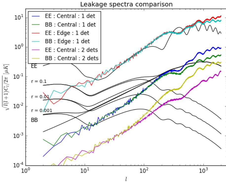
**Figure 16.**  $EE$  and  $BB$  spectra of leakage due to beam asymmetry and cross-polarization. The spectra are computed from the difference of the output CMB map with the input map. The effect of the additional asymmetry of the edge detectors is reflected in the increase in the leakage spectra as compared to the boresight detector. The leakage is decreased when using a pair of orthogonally polarized detectors due to better modulation of angles.
