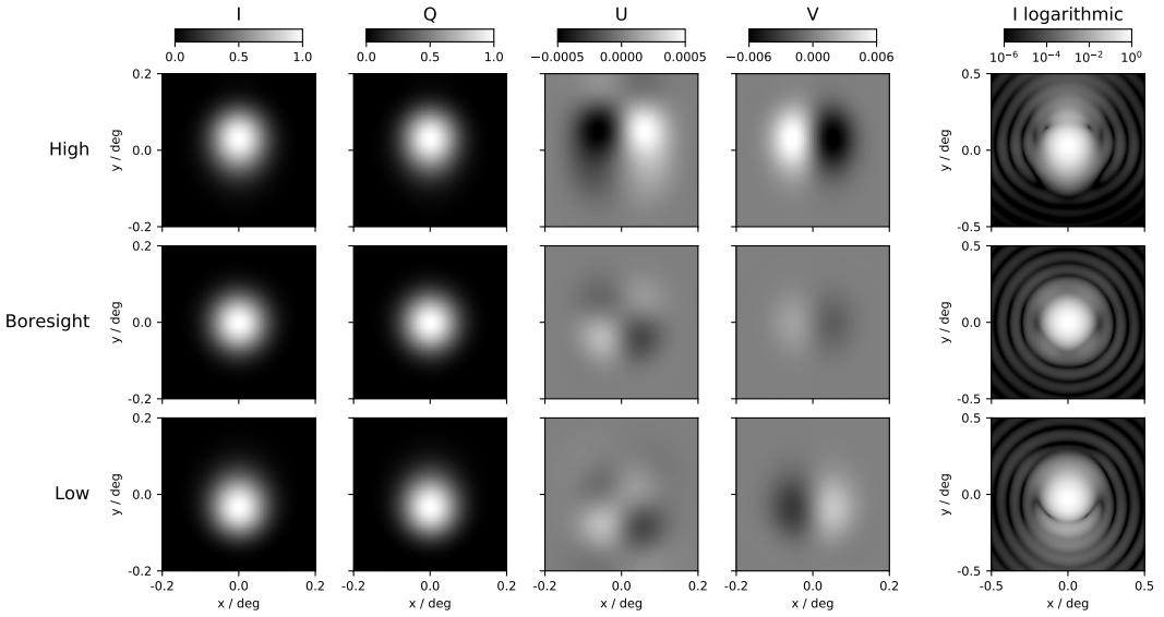
**Figure 14.** Simulated 145 GHz beams for the cross-Dragonian design of the *CORE* telescope. The three rows show the beams for the high, boresight, and low detectors (see text for details). The first 4 columns show the  $I$ ,  $Q$ ,  $U$ , and  $V$  Stokes parameters of the beams on a linear scale. The last column shows a wider view of the  $I$  Stokes parameter on a logarithmic scale. The Stokes parameters have been normalized to unity at the peak in intensity.
