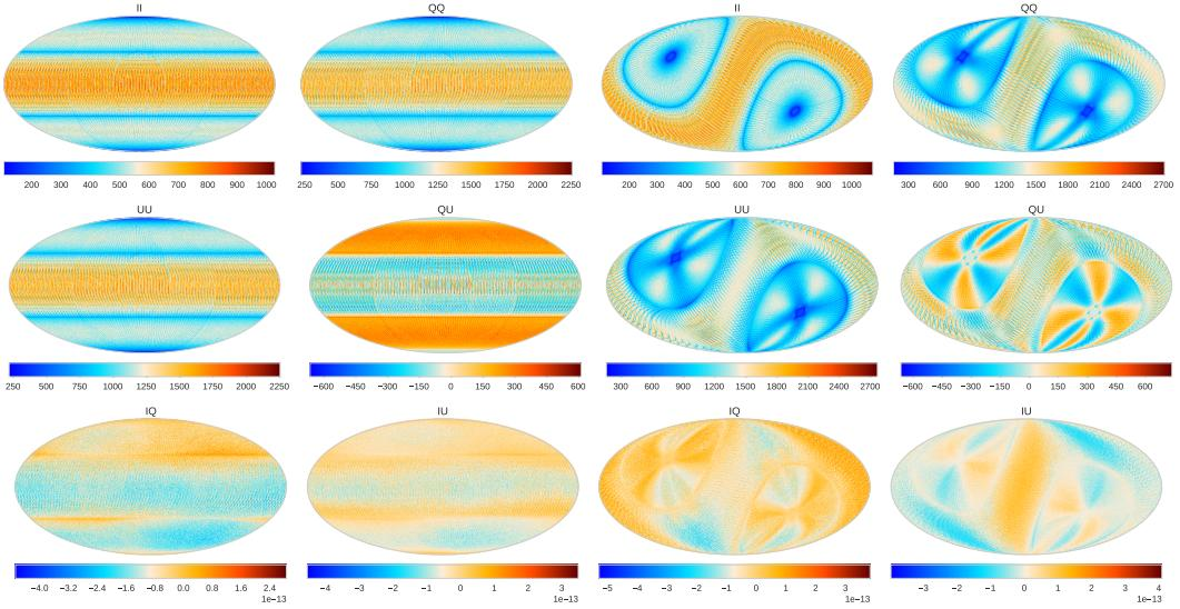
**Figure 3.** Elements of the white noise covariance matrix for a pair of boresight detectors displayed as maps in units of  $\mu K^2$ :  $II$  (top left),  $QQ$  (top right),  $UU$  (center left),  $QU$  (center right),  $IU$  (bottom left),  $IQ$  (bottom right). Coordinates are Ecliptic (left columns) and Galactic (right columns). Notice that  $IQ$  and  $IU$  correlations are very weak.
