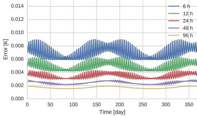
**Figure 22.** The uncorrelated statistical errors for the gains shown in the plot on the left of Fig. 21 in the case of a CMB-only sky for different lengths of the calibration period. The errors have been computed assuming diagonality for the gain covariance matrix, and they are therefore a lower bound. Both the short- and long-period fluctuations in the error are anticorrelated with the amplitude of the dipole signal; see the plot on the left of Fig. 19.
