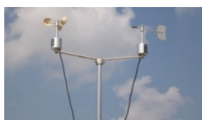
Figure 4.29 Vector Instruments Switching Porton Anemometer A100 and Encoder Windvane W200G
