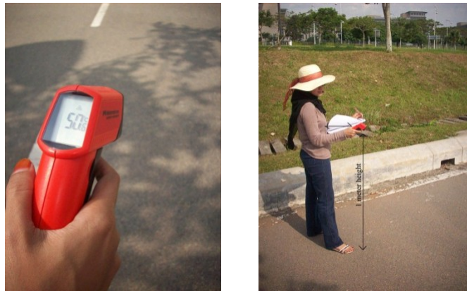
Figure 4.33 The reading taken from handheld Meteman IR608 Infrared Thermometer (left); and measurement procedure during measurement taken at 1m chest height
