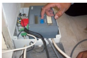
Figure 4.27 Eltek 1000 Series Squirrel data logger
