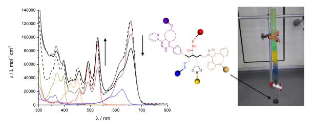
**Figure 5-39** Left: Absorption spectra (in grey after 4 h of reaction in DMA; black after 16 h in CHCl<sub>3</sub>) of pentad **5-64** normalized with arithmetic sum of dyes (dashed black) ADIBO-Py **5-2**, Y-Per **4-1**, R-PDI **4-2**, B-NDI **3-12**, B-Cy **5-20** on Y-Py unit (396 nm) in CHCl<sub>3</sub>; Right: Purification of **5-64** by GPC.
