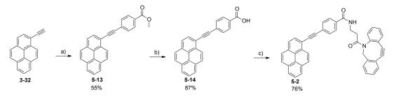
Scheme 5-4 Synthesis of ADIBO-ethynylpyrene 5-2; a) methyl-4-bromo-benzoate,  $[Pd(PPh_3)_2Cl_2]$ , CuI, NEt<sub>3</sub>, THF, 40 °C, 16 h; b) NaOH 2M (aq), THF/EtOH, rt, 3 h; c) ADIBO-amine 5-10, EDC.HCl, DMAP, CH<sub>2</sub>Cl<sub>2</sub>, rt, 20 h.
