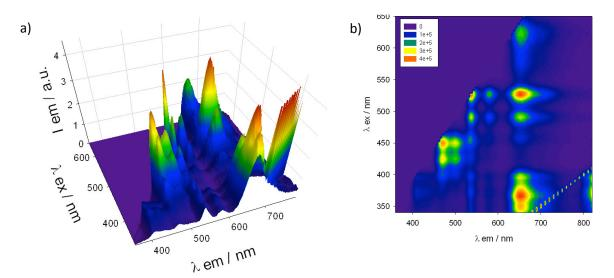
**Figure 5-31** a) Emission map for **5-56** in CHCl<sub>3</sub> at  $340 < \lambda_{exc} < 650$  nm. b) Emission contour map for **5-56**.
