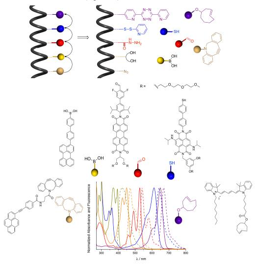
**Figure 5-1** Top: Schematic representation of the creation of the fully extended absorption range multichromophoric peptide; Bottom: Structure and normalized absorbance (solid line) and fluorescence emission (dashed line) of ADIBO-ethynylpyrene (green), Y-Per (orange), R-PDI (red), B-NDI (blue), B-Cy (purple) in DMF.
