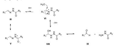
Scheme 2-13 Putative mechanism for the hydrolysis of acyl hydrazone.
