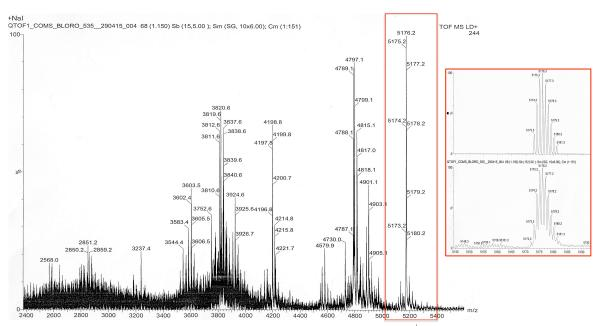
**Figure 3-16** MALDI-Tof analysis of peptide **3-37**; Inset: zoom of  $[M + Na]^+$  peak (bottom-right) compared with the calculated mass (top-right).
