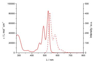
**Figure 3-11** Absorption (solid line) and fluorescence emission (dashed line) spectra ( $\lambda_{exc} = 495$  nm) of R-PDI **3-13** in DMF.
