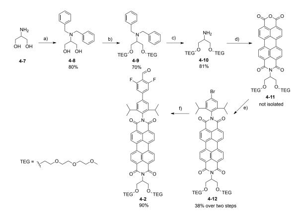
**Scheme 6-19** Synthesis of new R-PDI **4-2**; a) BnBr,  $K_2CO_3$ , EtOH, reflux, 3 h; b) NaH, TEG-OTs, THF, reflux, 20 h; c) H<sub>2</sub>, Pd/C, MeOH, rt, 20 h; d) *i*) PDA, Et<sub>3</sub>N, iPrOH/H<sub>2</sub>O, 120 °C, 10 d, *ii*) 5% HCl (aq), 120 °C, 10 min; e) 4-bromo-2,6-diisopropylaniline, propionic acid, MW irr, 140 °C, 7 h; f) 3,5-difluoro-4-formylphenyl boronic acid,  $K_2CO_3$ , [Pd(PPh<sub>3</sub>)<sub>4</sub>], dioxane/H<sub>2</sub>O, 80 °C, 20 h.
