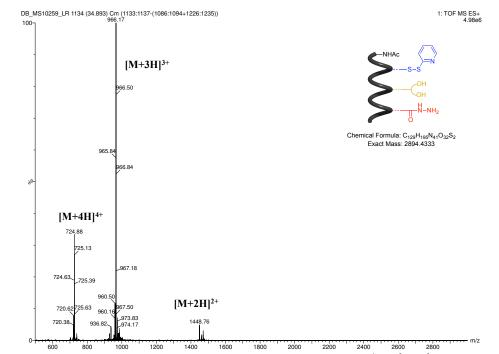
Figure 4-22 ESI-MS(Q-TOF) analysis of purified peptide 4-22 showing M<sup>4+</sup>, M<sup>3+</sup>, M<sup>2+</sup> multicharged ions.
