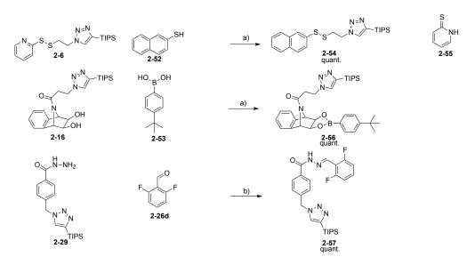
Scheme 2-22 Disulfide interchange, boronate and acyl hydrazone formation; a) THF, rt, 1 h; b) *m*-phenylene diamine, THF, rt, 1 h.
