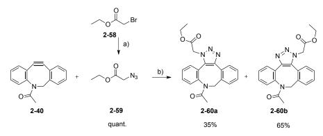
Scheme 6-9 Strain-promoted azide-alkyne cycloaddition; a) NaN<sub>3</sub>, H<sub>2</sub>O/acetone (1:3), 60 °C, 4 h; b) THF, rt, 1 h
