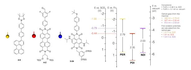
**Figure 4-6** Left: Structure of the dyes used to determine HOMO/LUMO energy levels by CV and absorption spectroscopy; Right: Frontier orbital potentials determined by cyclic voltammetry in DMF.
