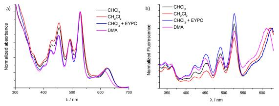
**Figure 5-23** a) Normalized absorption spectra (at 527 nm) of triad **5-48** in different media; b) excitation spectra of **5-48** normalized at the excitation maximum of B-NDI unit ( $\lambda_{em}$ =640 nm) in different media.
