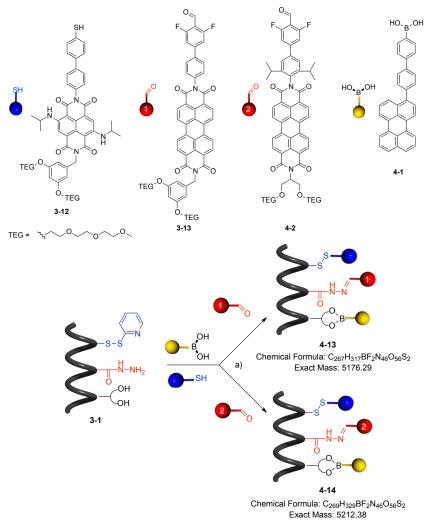
Scheme 4-3 Colored assembly with B-NDI 3-12, R-PDI 3-13 or 4-2 and Y-Per 4-1 on peptidic scaffold 3-1; a) *m*-PDA, DMF, rt, 4 h.
