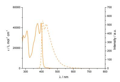
Figure 3-13 Absorption and fluorescence emission spectra ( $\lambda_{exc}$  = 398 nm) of Y-Py 3-14 in DMF.
