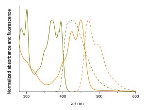
**Figure 5-3** Normalized absorbance (solid line) and fluorescence emission (dashed line) of ADIBO-perylene **5-1** ( $\lambda_{exc}$  = 423 nm, orange) and ADIBO-ethynylpyrene **5-2** ( $\lambda_{exc}$  = 371 nm, green) in DMF.
