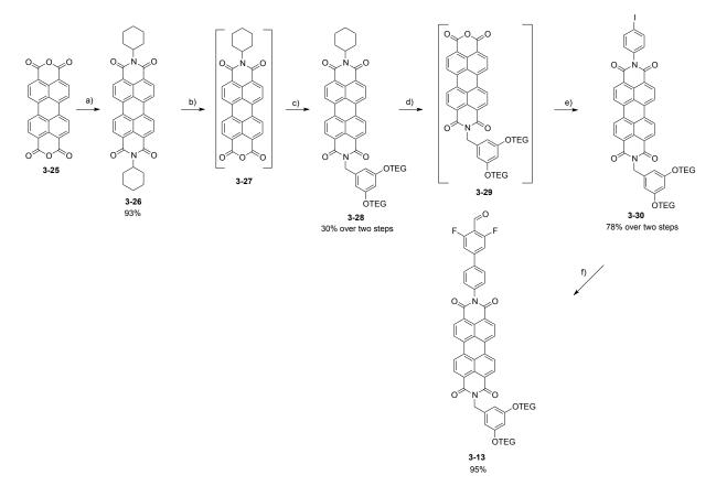
Scheme 3-9 Synthesis of R-PDI 3-13; a) cyclohexylamine, 140 °C, 15 h; b) *i*) KOH, iPrOH/H<sub>2</sub>O (6:1), 80 °C, 3 h, *ii*) AcOH, rt, 15 min; c) 3-17, imidazole, toluene/DMF (6:1), 110 °C, 16 h; d) *i*) KOH, iPrOH/H<sub>2</sub>O (6:1), 80 °C, 3 h, *ii*) AcOH, rt, 15 min; e) iodo-aniline, imidazole, toluene/DMF (6:1), 110 °C, 16 h; f) 2,6-difluoro-4-formylphenylboronic acid,  $K_2CO_3$ , [Pd(PPh<sub>3</sub>)<sub>4</sub>], dioxane/H<sub>2</sub>O (7:1).
