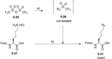
Scheme 6-27 Synthesis of Fmoc-Nle(N<sub>3</sub>)-OH 5-21; a) NaN<sub>3</sub>,  $H_2O/CH_2Cl_2$ , rt, 2 h; b) NaHCO<sub>3</sub>, CuSO<sub>4</sub>.5H<sub>2</sub>O, H<sub>2</sub>O/MeOH (1:2), rt, 18 h.
