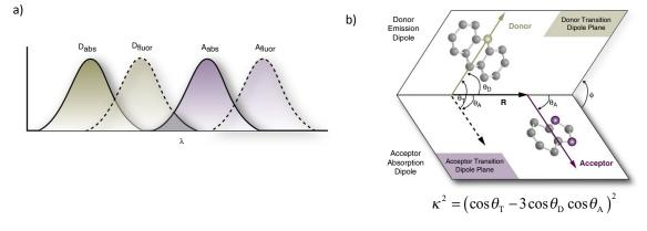
**Figure 1-6** a) Representation of the normalized spectral overlap between the donor emission and the acceptor absorption; b) Transition dipole orientation and schematic representation of the angles used to calculate  $k^2$ . Adapted with permission from reference 5a. Copyright (2017) American Chemical Society. <sup>[5a]</sup>
