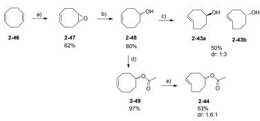
Scheme 2-20 Synthesis of *trans*-cyclooctene 2-43 and 2-44; a) *m*-CPBA, CHCl<sub>3</sub>, 0 °C to rt, 12 h; b) LiAlH<sub>4</sub>, THF, 0 °C to 70 °C, 4 h; c) methyl benzoate, *hv* 254 nm, Et<sub>2</sub>O/hexane (9:1), AgNO<sub>3</sub>/SiO<sub>2</sub>, 10 × 30 min; d) acetic anhydride, pyridine, CH<sub>2</sub>Cl<sub>2</sub>, 20 h, 40 °C, e) methyl benzoate, *hv* 254 nm, Et<sub>2</sub>O/hexane (1:9), AgNO<sub>3</sub>/SiO<sub>2</sub>, 10 × 30 min.
