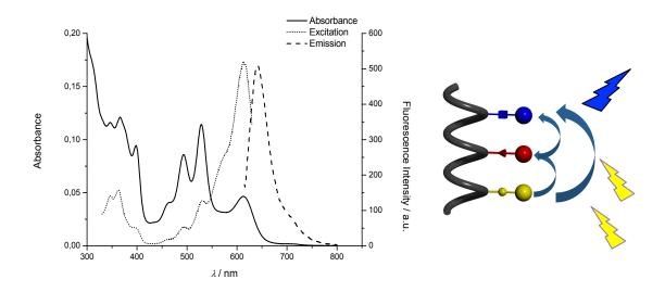
**Figure 3-20** Left: Absorption (solid line), emission (long-dashed line,  $\lambda_{exc}$  =609 nm), and excitation profiles (short-dashed line,  $\lambda_{em}$  = 640 nm) for peptide **3-37** in DMF, C = 2  $\mu$ M. Right: Schematic representation of ET from R-PDI to B-NDI and from Y-Py to B-NDI either by direct or stepwise ET cascade.
