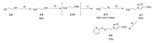
Scheme 2-7 Synthesis of pyridine disulfide 2-6; a) TrtCl, THF, 50 °C, 4 h; b) MsCl, Et<sub>3</sub>N, CH<sub>2</sub>Cl<sub>2</sub>, 0 °C to rt, 2 h; c) NaN<sub>3</sub>, DMF, 70 °C, 3 h; d) TIPS acetylene, CuSO<sub>4</sub>·5H<sub>2</sub>O, Na ascorbate, DMF/H<sub>2</sub>O (4:1), rt, 16 h; e) *i*) TFA, TIS, CH<sub>2</sub>Cl<sub>2</sub>, rt, 1 h, *ii*) 2,2'-dipyridyl disulfide, DIEA, CH<sub>2</sub>Cl<sub>2</sub>, rt, 1 h.
