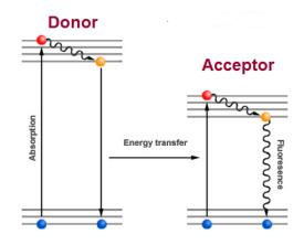
Figure 1-5 Jablonski diagram of FRET.<sup>[12]</sup>
