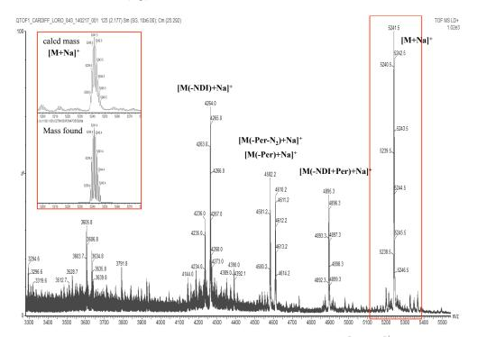
**Figure 5-15** MALDI-Tof analysis of purified peptide **5-45**; inset: Zoom of  $[M+Na]^+$  peak (top) compared with calculated mass (bottom).
