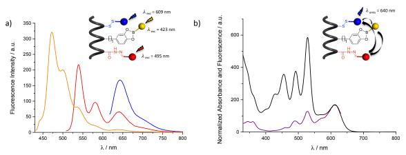
**Figure 4-34** a) Fluorescence emission spectra of YRB peptide **4-42** at ( $\lambda_{exc}$ ) 423 nm (yellow), 495 nm (red), 609 nm (blue) to determine ET efficiencies following the method 1:  $\Phi_{ET} = QY^*_{B-NDI}/QY_{B-NDI}$ ; b) Normalized absorption (black) and fluorescence excitation (purple) spectra of YRB peptide **4-42** ( $\lambda_{em}$ =640 nm) for the method 2:  $\Phi_{ET} = Ex_D/A_D$ .
