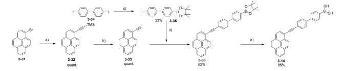
**Scheme 3-10** Synthesis of Y-Py **3-14**; a) TMS-acetylene,  $[Pd(PPh_3)_2Cl_2]$ , CuI, NEt<sub>3</sub>, 70 °C, 20 h; b) K<sub>2</sub>CO<sub>3</sub>, MeOH/THF (1:1), rt, 20 h; c) KOAc, B<sub>2</sub>Pin<sub>2</sub>,  $[PdCl_2(dppf)]$ , DMSO, 80 °C, 20 h; d)  $[Pd(PPh_3)_2Cl_2]$ , CuI, NEt<sub>3</sub>, THF, 40 °C, 6 h; e) HCl (aq, 2M)/THF (1:2), rt, 40 h.
