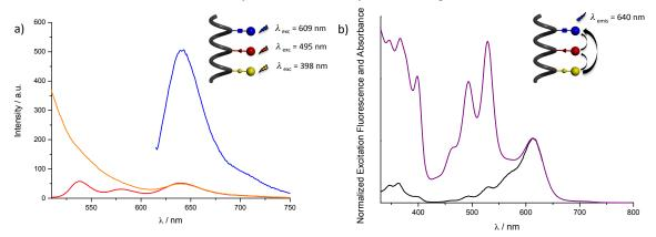
**Figure 3-21** a) Fluorescence emission spectra of **3-37** at ( $\lambda_{exc}$ ) 398 nm, 495 nm, 609 nm in DMF (C = 2  $\mu$ M). b) Normalized absorption (in purple) and fluorescence excitation (in black) spectra ( $\lambda_{emis}$  = 640 nm) of YRB peptide **3-37** in DMF.
