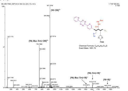
**Figure 5-37** ESI-HRMS(Q-Tof) analysis of peptide **5-62** showing  $[M+2H]^{2+}$ ,  $[M+H]^{+}$  and fragmented ions.
