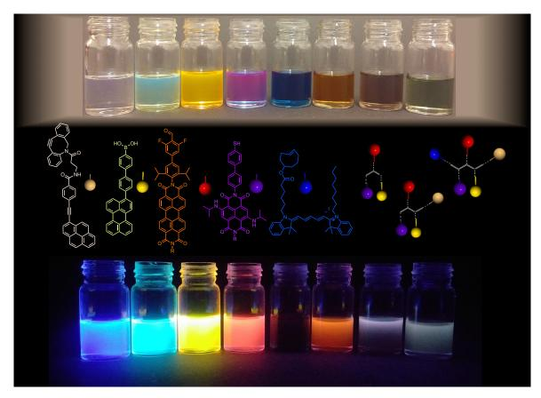
**Figure 5-44** Pictures of solutions of (from left to right) free dyes Y-Py **5-2**, Y-Per **4-1**, R-PDI **4-2**, B-NDI **3-12**, B-Cy **5-3**, triad **5-48**, tetrad **5-56**, pentad **5-64** under visible (top), UV light ( $\lambda_{exc} = 254$  nm) (bottom).
