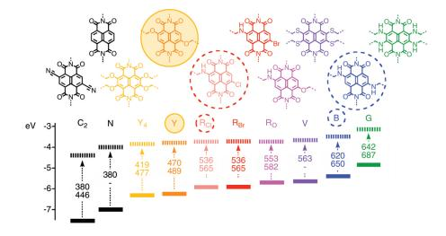
**Figure 3-9** Core substituted naphtalenediimides: "A rainbow collection" with indication of HOMO (bold) and LUMO (dashed) energies in eV against vacuum and maximal absorption (top) and emission wavelength (bottom) in nm. Reprinted from reference 15b with permission. Copyright (2009) American Chemical Society.<sup>[15b]</sup>
