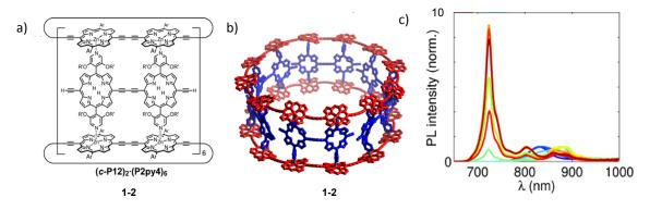
Figure 1-10 a, b) Structure of ring-dimer-ring complex 1-2, Ar = 3,5-bis(trihexylsilyl)phenyl, R' = dodecyl; c) Steady state emission titrations of the associated complex (spectrum in blue) which is dissociated upon addition of a competing ligand (spectrum of fully dissociated complex in red with 6 equiv. of ligand) ( $\lambda_{exc} = 450$  1 c  $1^{-1}$  c  $1^{-1}$
