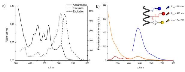
**Figure 4-10** a) Absorption (solid line), Emission ( $\lambda_{exc} = 609 \text{ nm}$ ) (long-dashed line), Excitation ( $\lambda_{em} = 640 \text{ nm}$ ) (short dashed line) spectra of YRB peptide **4-13**; b) Fluorescence emission spectra of YRB peptide upon selective excitation of B-NDI ( $\lambda_{exc} = 609 \text{ nm}$ ), R-PDI ( $\lambda_{exc} = 495 \text{ nm}$ ), Y-Per ( $\lambda_{exc} = 423 \text{ nm}$ ) in DMF.
