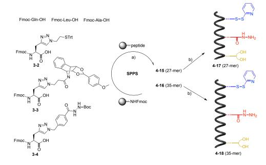
Scheme 4-3 Peptidic scaffold 4-17 and 4-18 synthesis; a) SPPS: *i*) Fmoc deprotection: 20% piperidine in DMF, rt,  $3 \times 6$  min; *ii*) AA coupling: Fmoc-AA-OH, HATU, DIEA, DMF/NMP, rt, 25 min; *iii*) Ac<sub>2</sub>O/pyridine/NMP (1:2:2),  $2 \times 15$  min; *iv*) TFA/TIS/H<sub>2</sub>O/EDT (94:1:2.5:2.5), rt, 2 h; b) 2,2'-dipyridyl disulfide, DIEA, DMF, 1 h.
