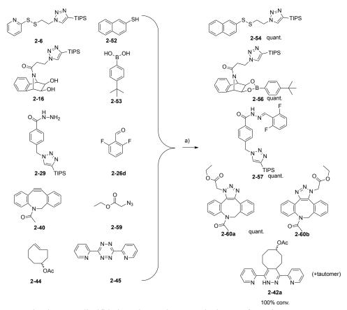
Scheme 2-28 Simultaneous disulfide interchange, boronate, hydrazone formation, SPAAC, IEDDA; a) *m*-PDA, THF, rt, 1 h.
