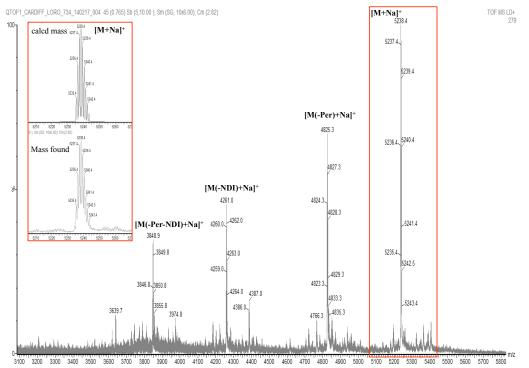
**Figure 4-23** MALDI-TOF analysis of purified peptide **4-23**; Inset: Zoom of  $[M+Na]^+$  peak (bottom) compared with calculated mass  $[M+Na]^+$  (top).
