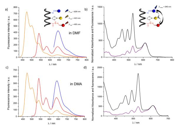
**Figure 4-38** Fluorescence emission spectra of YRB peptide **4-23** at ( $\lambda_{exc}$ ) 423 nm (yellow), 495 nm (red), 609 nm (blue) to determine ET efficiency following the method 1:  $\Phi_{ET} = QY^*_{B-NDI}/QY_{B-NDI}$  in a) DMF and c) DMA; Normalized absorption and fluorescence excitation spectra of YRB peptide **4-23** ( $\lambda_{em} = 640$  nm) for the method 2:  $\Phi_{ET} = Ex_D/A_D$  in b) DMF and d) DMA.
