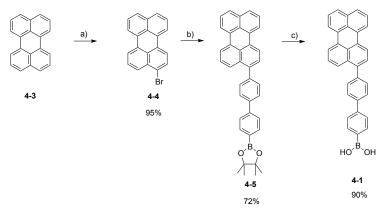
Scheme 4-1 Synthesis of Y-Per 4-1; a) NBS, THF, rt, 24 h; b) 4,4'-biphenyldiboronic acid bis(pinacol)ester,  $K_2CO_3$ ,  $[Pd(PPh_3)_4]$ , dioxane/H<sub>2</sub>O, 85 °C, 3 h; c) *i*) NaIO<sub>4</sub>, THF/H<sub>2</sub>O (4 :1), rt, 1 h 30, *ii*) HCl (1M), rt, 20 h.
