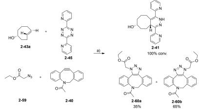
Scheme 2-27 Simultaneous IEDDA and SPAAC reactions; a) THF, rt, 1 h.
