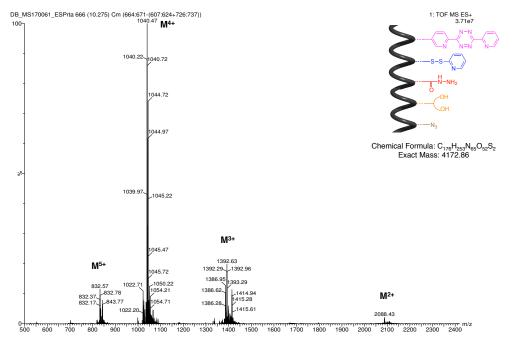
Figure 5-33 LC-ESI-MS(Q-Tof) analysis of crude peptide 5-60 showing  $[(M+2)+2H]^{2+}$ ,  $[(M+2)+3H]^{3+}$ ,  $[(M+2)+4H]^{4+}$ .
