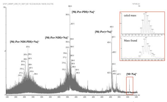
**Figure 4-8** MALDI-TOF analysis of purified peptide **4-14**; Inset: Zoom of  $[M+Na]^+$  peak (bottom) compared with calculated mass (top).
