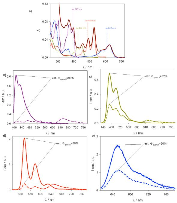
**Figure 6-48** a) Absorption and emission spectra of tetrad **5-56** and free dyes (dashed line) used to evaluate the emission quenching on tetrad **5-56** (dashed lines): b) Y-Py ( $\lambda_{exc}$ =393 nm), c) Y-Per ( $\lambda_{exc}$ =427 nm), d) R-PDI ( $\lambda_{exc}$ =487 nm), d) B-NDI ( $\lambda_{exc}$ =610 nm).
