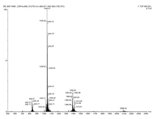
**Figure 6-43** LC-ESI-MS(Q-Tof) analysis of crude peptide **5-60** showing  $[(M+2)+2H]^{2+}$ ,  $[(M+2)+3H]^{3+}$ ,  $[(M+2)+4H]^{4+}$ .
