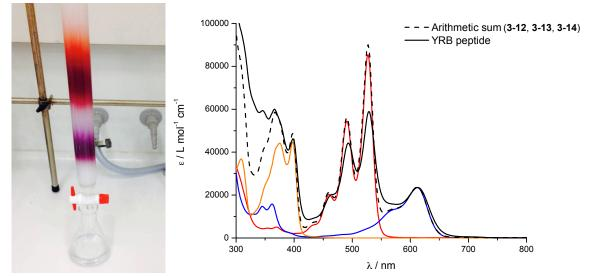
Figure 3-15 Left) Purification of peptide 3-37 by Gel Permeation Chromatography; Right) Normalized absorption spectra of peptide 3-37 with arithmetic sum of dyes 3-12, 3-13 and 3-14 absorption on B-NDI (612 nm) in DMF.
