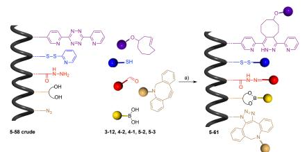
Scheme 5-16 Chromophoric assembly of ADIBO-Py 5-2, R-PDI 4-2, Y-Per 4-1, B-NDI 3-12, TCO-Cy 5-3 within crude peptide 5-58; a) *m*-PDA, DMA, 4 h, rt, 3 h, 40 °C.
