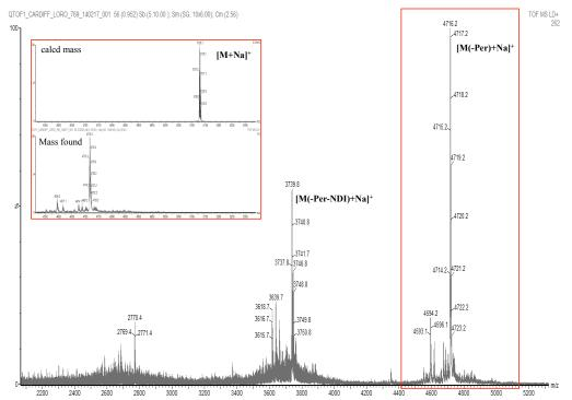
**Figure 4-31** MALDI-TOF analysis of purified peptide **4-42**; Inset: Zoom of  $[M(-boronate)+Na]^+$  peak (bottom) compared with calculated mass  $[M+Na]^+$  (top).
