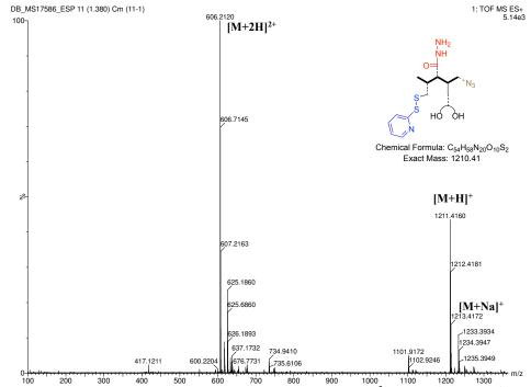
Figure 5-27 ESI-MS(Q-Tof) analysis of peptide 5-55 showing  $[M+2H]^{2+}$ ,  $[M+H]^{+}$ ,  $[M+Na]^{+}$ .
