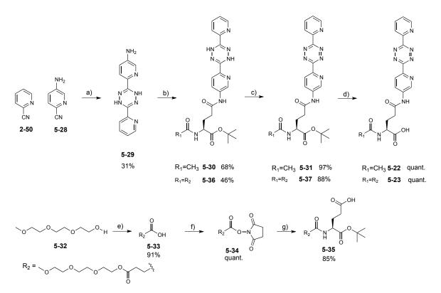
Scheme 6-28 Syntheses of tetrazine containing aa 5-22 and 5-23; a) hydrazine hydrate, 90 °C, 12 h; b)  $R_2(CO)$ -Glu-OtBu, EDC.HCl, DMAP,  $CH_2Cl_2$ , rt, 20 h; c) PIDA,  $CH_2Cl_2$ , rt, 1.5 h; d) TFA,  $CH_2Cl_2$ , rt, 2 h; e) succinic anhydride, DMAP,  $CH_2Cl_2$ , rt, 20 h; f) *N*-hydroxysuccinimide, EDC.HCl, DMAP,  $CH_2Cl_2$ , rt, 20 h; g) H-Glu-OtBu, DIEA, DMF, rt, 16 h.
