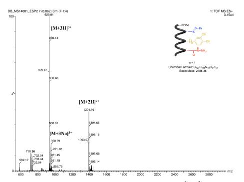
Figure 4-29 ESI-MS(Q-TOF) analysis of purified peptide 4-40 showing M<sup>3+</sup>, M<sup>2+</sup> multicharged ions.
