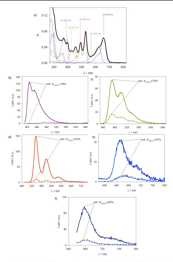
**Figure 6-49** a) Absorption and emission spectra of pentad **5-64** and free dyes (dashed line) used to evaluate the emission quenching on pentad **5-64** (dashed lines): b) Y-Py ( $\lambda_{exc}$ =393 nm), c) Y-Per ( $\lambda_{exc}$ =423 nm), d) R-PDI ( $\lambda_{exc}$ =486 nm), d) B-NDI ( $\lambda_{exc}$ =566 nm), e) B-Cy ( $\lambda_{exc}$ =658 nm).
