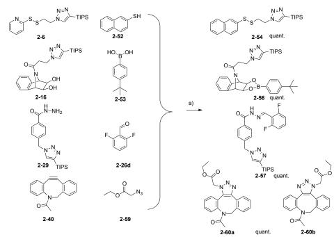
Scheme 2-25 Simultaneous disulfide interchange, boronate, acyl hydrazone formation and SPAAC; a) *m*-PDA, THF, rt, 1 h.
