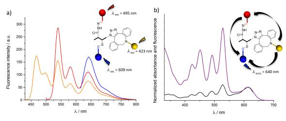
**Figure 5-21** a) Fluorescence emission spectra of YRB peptide **5-48** in DMA at ( $\lambda_{exc}$ ) 423 nm (yellow), 495 nm (red), 609 nm (blue) to determine ET efficiencies following method 1:  $\Phi_{ET} = QY *_{B-NDI}/QY_{B-NDI}$ ; b) Normalized absorption (black) and fluorescence excitation (purple) spectra of **5-48** in DMA ( $\lambda_{em}$ =640 nm) for method 2:  $\Phi_{ET} = Ex_D/A_D$ .
