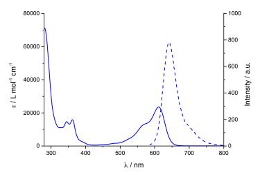
**Figure 3-10** Absorption (solid line) and fluorescence emission (dashed line) spectra ( $\lambda_{exc} = 580$  nm) of B-NDI **3-12** in DMF.
