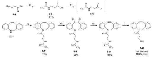
**Scheme 5-2** Synthesis of ADIBO-amine **5-10**; a) ethyltrifluoroacetate, NEt<sub>3</sub>, MeOH, rt, 24 h; b) oxalyl chloride, DMF (cat),  $CH_2Cl_2$ , rt, 2 h; c) **5-6**, pyridine,  $CH_2Cl_2$ , rt, 1 h; d) pyridinium tribromide,  $CH_2Cl_2$ , rt, 18 h; e) *t*BuOK, THF, rt, 1 h; f)  $K_2CO_3$ , MeOH/H<sub>2</sub>O, rt, 18 h.<sup>[1b]</sup>
