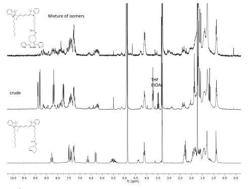
**Figure 6-20** <sup>1</sup>H NMR of TCO-cyanine **5-3** (bottom), crude material showing full conversion into product and excess of tetrazine (middle), tetrazine ligation product **5-20** (top) in MeOD- $d_4$
