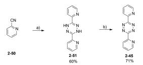
Scheme 2-21 Synthesis of dipyridyl-s-tetrazine 2-45; a) hydrazine hydrate, 90 °C, 12 h; b) DDQ, toluene, 110 °C, 12 h.
