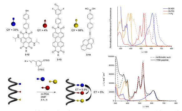
Figure 3-28 Top left: three color emitters: B-NDI 3-12, R-PDI 3-13, Y-Py 3-14; top right: normalized absorption (solid) and fluorescence (dashed) spectra of the 3 color emitters; bottom left: colored assembly on the scaffold giving YRB peptide; bottom right: absorption spectrum of YRB peptide 3-37 normalized with arithmetic sum of the absorption spectra of color emitters 3-12, 3-13, 3-14 on B-NDI.
