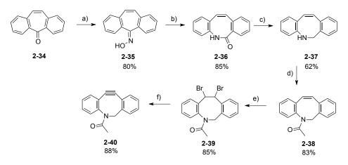
Scheme 6-4 Synthesis of ADIBO 2-40; a) hydroxylamine.HCl, pyridine, 120 °C, 20 h; b) polyphosphoric acid, 125 °C, 1 h; c) LiAlH<sub>4</sub>, Et<sub>2</sub>O, 40 °C, 18 h; d) AcCl, pyridine,  $CH_2Cl_2$ , rt, 1 h; e) pyridinium tribromide,  $CH_2Cl_2$ , rt, 18 h; f) tBuOK, THF, rt, 1 h.
