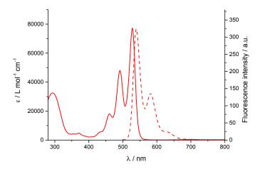
**Figure 4-5** Absorption (solid line) and fluorescence emission (dashed line) ( $\lambda_{exc}$ =495 nm) spectra of R-PDI **4-2** recorded in DMF.
