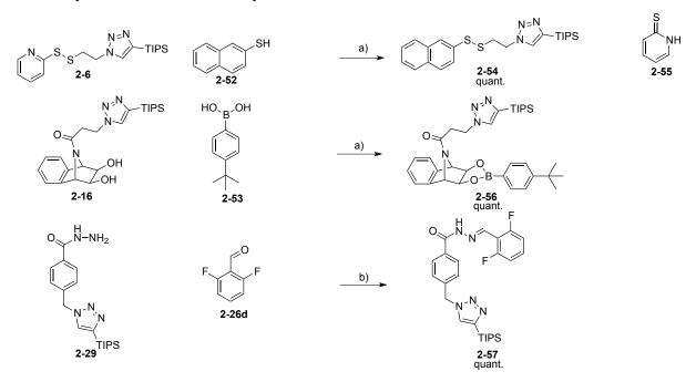
Scheme 6-7 Disulfide exchange, boronate and acyl hydrazone formation; a) THF, rt, 1 h; b) *m*-phenylenediamine, THF, rt, 1 h.
