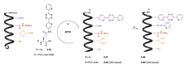
Scheme 5-15 Synthesis of peptidic scaffolds 5-58 and 5-60; a) SPPS: *i*) Fmoc deprotection: 20% piperidine in DMF, rt,  $3 \times 6$  min; *ii*) AA coupling: Fmoc-AA-OH, HATU, DIEA, DMF/NMP, rt, 25 min or 1 h for last coupling with tetrazine containing aa; *iii*) TFA/TIS/H<sub>2</sub>O (95:2.5:2.5), rt, 2 h; b) 2,2'-dipyridyl disulfide, DIEA, DMF, 1 h.
