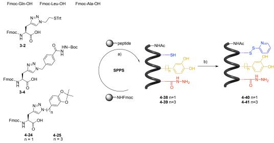
**Scheme 4-9** Peptidic scaffold synthesis; a) SPPS: i) Fmoc deprotection: 20% piperidine in DMF, rt,  $3 \times 6$  min; ii) AA coupling: Fmoc-AA-OH, HATU, DIEA, DMF/NMP, rt, 25 min; iii) Ac<sub>2</sub>O/pyridine/NMP (1:2:2),  $2 \times 15$  min; iv) TFA/TIS/H<sub>2</sub>O/EDT (94:1:2.5:2.5), rt, 2 h; b) 2,2'-dipyridyl disulfide, DIEA, DMF, 1 h.
