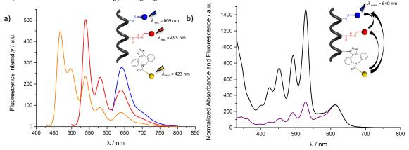
**Figure 5-17** a) Fluorescence emission spectra of RYB peptide **5-45** at  $(\lambda_{exc})$  423 nm (yellow), 495 nm (red), 609 nm (blue) in DMA to determine ET efficiencies following method 1:  $\Phi_{ET} = QY^*_{B-NDI}/QY_{B-NDI}$ ; b) Normalized absorption (black) and fluorescence excitation (purple) spectra of YRB peptide **5-45** ( $\lambda_{em}$ =640 nm) in DMA for method 2:  $\Phi_{ET} = Ex_D/A_D$ .
