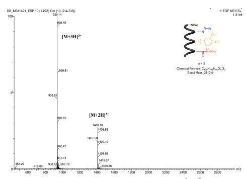
Figure 4-30 ESI-MS(Q-TOF) analysis of purified peptide 4-41 showing  $M^{3+}$ ,  $M^{2+}$  multicharged ions.
