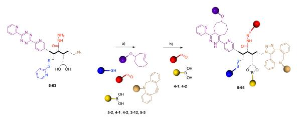
**Scheme 5-18** Chromophoric assembly of ADIBO-Py **5-2**, R-PDI **4-2**, Y-Per **4-1**, B-NDI **3-12**, B-Cy **5-3** within peptide **5-63**; a) *m*-PDA, DMA, 2 h, rt, 2 h, 40 °C; b) *m*-PDA, CHCl<sub>3</sub>, 16 h, rt.
