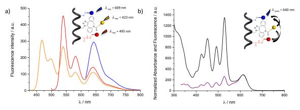
**Figure 5-16** a) Fluorescence emission spectra of RYB peptide **5-44** at ( $\lambda_{exc}$ ) 423 nm (yellow), 495 nm (red), 609 nm (blue) in DMA to determine ET efficiencies following method 1:  $\Phi_{ET} = QY^*_{B-NDI}/QY_{B-NDI}$ ; b) Normalized absorption (black) and fluorescence excitation (purple) spectra of YRB peptide **5-44** ( $\lambda_{em}$ =640 nm) in DMA for method 2:  $\Phi_{ET} = Ex_D/A_D$ .
