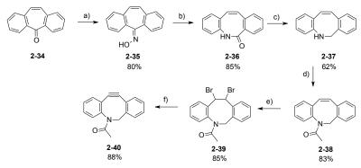
**Scheme 2-17** Synthesis of ADIBO **2-40**; a) hydroxylamine.HCl, pyridine, 120 °C, 20 h; b) polyphosphoric acid, 125 °C, 1 h; c) LiAlH<sub>4</sub>, Et<sub>2</sub>O, 40 °C, 18 h; d) AcCl, pyridine, CH<sub>2</sub>Cl<sub>2</sub>, rt, 1 h; e) pyridinium tribromide, CH<sub>2</sub>Cl<sub>2</sub>, rt, 18 h; f) *t*BuOK, THF, rt, 1 h.<sup>[39]</sup>
