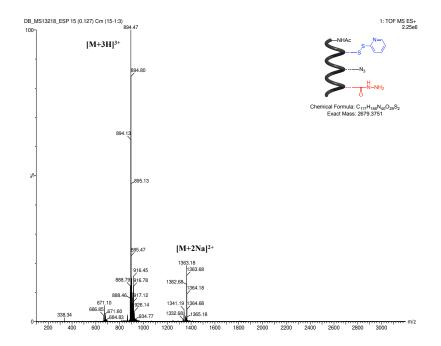
Figure 5-11 ESI-MS(Q-Tof) analysis of purified peptide 5-42 showing [M+3H]<sup>3+</sup>, [M+2Na]<sup>2+</sup>.
