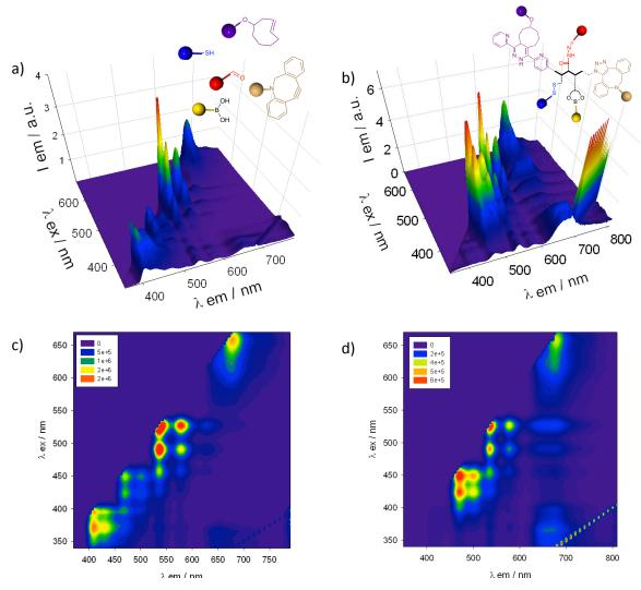
**Figure 5-41** Comparison between emission map (a,b) and contour map (c,d) of isoabsorbing solutions of a, c) mixture of 5 chromophores **5-2, 4-1, 4-2, 3-12, 5-3** and b, d) peptide **5-64** in anhydrous CHCl<sub>3</sub>;  $340 < \lambda_{exc} < 670$  nm.
