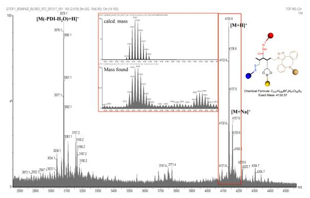
**Figure 5-29** MALDI-Tof analysis of peptide **5-56**; Inset: Zoom of  $[M+H]^+$  and  $[M+Na]^+$  peaks (bottom) compared with calculated mass  $[M+H]^+$  (top).
