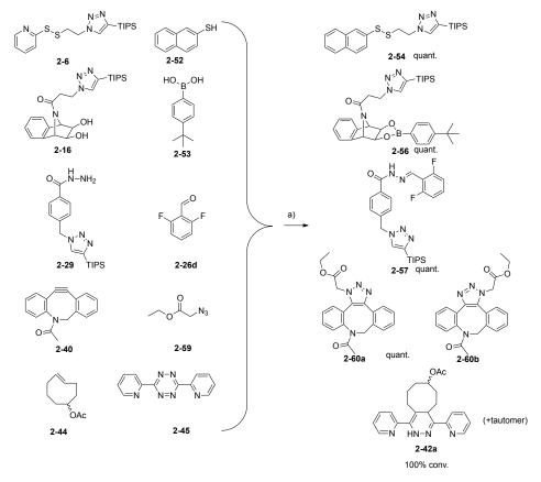
**Scheme 6-13** Simultaneous disulfide interchange, boronate, acyl hydrazone formation, SPAAC and IEDDA; a) *m*-phenylene diamine (*m*-PDA), THF, rt, 1 h.
