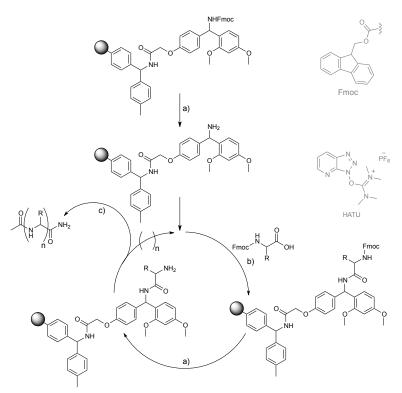
Scheme 3-5 General procedure of Solid Phase Peptide Synthesis in Fmoc/*t*Bu strategy (Fmoc/*t*Bu-SPPS); a) *i*) Fmoc deprotection: 20% piperidine in DMF,  $3 \times 4 \min$ , *ii*) DMF washing; b) *i*) HATU, DIEA, DMF, NMP, 25 min, *ii*) DMF washing c) *i*) Ac<sub>2</sub>O/pyridine/NMP (1:2:2),  $2 \times 15 \min$ ; *ii*) TFA/TIS/H<sub>2</sub>O/EDT, 94:1:2.5:2.5, 2 h.
