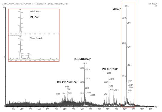
**Figure 4-36** MALDI-TOF analysis of purified peptide **4-23**; Inset: Zoom of  $[M+Na]^+$  peak (bottom) compared with calculated mass  $[M+Na]^+$  (top).
