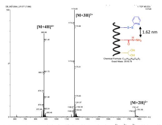
Figure 4-14 ESI-MS(Q-TOF) analysis of purified peptide 4-17 showing M<sup>4+</sup>, M<sup>3+</sup>, M<sup>2+</sup> multicharged ions.
