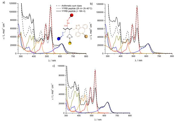
Figure 5-28 Absorption spectra of YYRB tetrad 5-56 normalized with arithmetic sum of chromophores ADIBO-Py 5-2, Y-Per 4-1, R-PDI 4-2, B-NDI 3-12 on B-NDI following a) one-pot approach in DMA; b) stepwise approach in DMA; c) in CHCl<sub>3</sub>.
