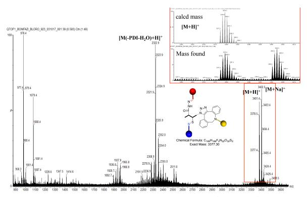
**Figure 5-20** MALDI-Tof analysis of peptide **5-48**; Inset: Zoom of  $[M+H]^+$  and  $[M+Na]^+$  peak (bottom) compared with calculated mass  $[M+H]^+$  (top).
