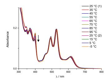
Figure 3-19 Absorption spectra of peptide 3-37 in DMF (3.2  $\mu$ M) at different temperatures. The arrow indicates changes upon increasing temperature.
