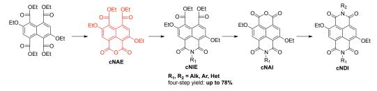
Scheme 3-7 Sequential methodology for the preparation of unsymmetrical cNDI.<sup>[16]</sup>
