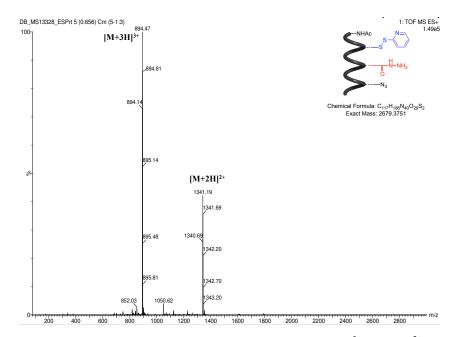
Figure 5-12 ESI-MS(Q-Tof) analysis of purified peptide 5-43 showing  $[M+3H]^{3+}$ ,  $[M+2H]^{2+}$ .
