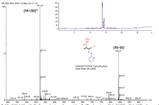
Figure 5-18 ESI-MS (Q-Tof) analysis of peptide 5-47 showing  $[M+2H]^{2+}$ ,  $[M+H]^+$ ; Inset: HPLC chromatogram of crude material 5-47.
