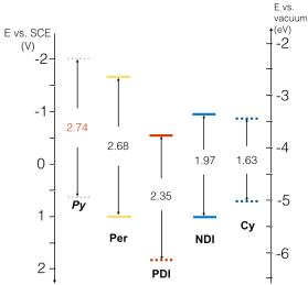
Figure 5-7 Frontier orbital potentials determined by cyclic voltammetry in  $CH_2Cl_2$ . Data for Py were taken from literature for a similar molecule.<sup>[12]</sup>
