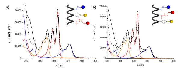
**Figure 4-24** Absorption spectrum of a) RYB peptide **4-23** (black solid line) and b) YRB peptide **4-14** (black solid line) normalized on B-NDI with arithmetic sum (dashed line) of absorption of dyes B-NDI (in blue), R-PDI (in red), Y-Per (in yellow) in DMF.
