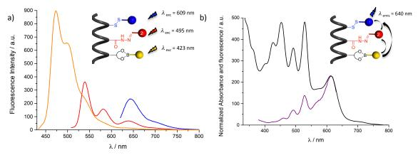
**Figure 4-11** a) Fluorescence emission spectra of YRB peptide 4-14 at ( $\lambda_{exc}$ ) 423 nm (yellow), 495 nm (red), 609 nm (blue) in DMF to determine ET efficiency following the first method:  $\Phi_{ET} = QY^*_{B-NDI}/QY_{B-NDI}$ ; b) Normalized absorption and excitation spectra ( $\lambda_{em}$ =640 nm) in DMF for the second method:  $\Phi_{ET} = Ex_D/A_D$ .
