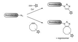
Figure 2-4 Bioorthogonal cycloaddition of azides and alkynes catalyzed by Cu<sup>1</sup> or promoted by strain.<sup>[18a]</sup>
