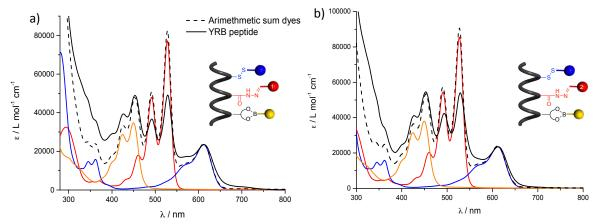
Figure 4-9 Absorption spectra of a) YRB peptide 4-13 (solid black line) and b) YRB peptide 4-14 (solid black line) normalized with arithmetic sum (dashed line) of absorption of dyes B-NDI 3-11, R-PDI 3-12 or 4-2, Y-Per 4-1 in DMF on B-NDI unit.
