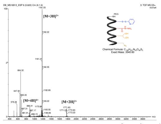
Figure 5-24 ESI-MS(Q-Tof) analysis of purified peptide 5-52 showing  $[M+2H]^{2+}$ ,  $[M+3H]^{3+}$ ,  $[M+4H]^{4+}$ .
