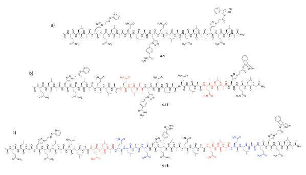
Figure 4-13 Structures of peptides a) 3-1, b) 4-17, c) 4-18 in which receptor sites are separated by 1.08 nm, 1.62 nm and 2.16 nm respectively.
