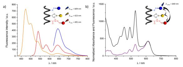
**Figure 4-25** a) Fluorescence emission spectra of RYB peptide **4-23** at ( $\lambda_{exc}$ ) 423 nm (yellow), 495 nm (red), 609 nm (blue) to determine ET efficiencies following the method 1:  $\Phi_{ET} = QY^*_{B-NDI}/QY_{B-NDI}$ ; b) Normalized absorption (black) and fluorescence excitation (purple) spectra of RYB peptide **4-23** ( $\lambda_{em}$ =640 nm) for the method 2:  $\Phi_{ET} = Ex_D/A_D$ .
