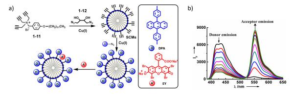
**Figure 1-16** a) Preparation of the artificial antenna based on surface-cross-linked micelles (SCM); b) Fluorescence emission spectra ( $\lambda_{exc} = 375$  nm) of DPA-SCM in black ( $C_D = 23 \mu$ M) upon addition of the acceptor EY ( $C_A = 0, 0.08, 0.17, 0.33, 0.5, 0.67, 0.84, 1, 1.17, 1.34 \mu$ M) in green for highest C<sub>A</sub> in THF. Adapted with permission from reference 30. Copyright (2015) American Chemical Society.<sup>[33]</sup>
