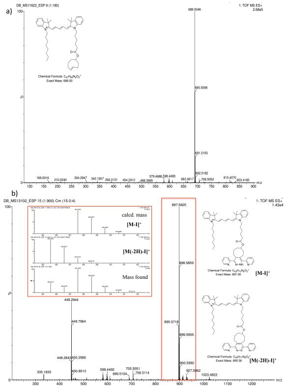
**Figure 5-5** ESI-HRMS(Q-Tof) analyses of a) TCO-cyanine **5-3**; b) cyanine tetrazine ligation product **5-20**; inset: zoom of monocharged peak showing mixture between  $[M-1]^+$  and  $[M(-2H)-1]^+$ .
