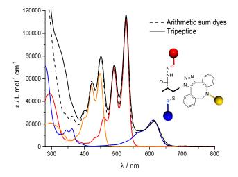
Figure 5-19 Absorption spectrum of triad 5-48 normalized with arithmetic sum of dyes ADIBO-Per 5-1, R-PDI 4-2 and B-NDI 3-12 on B-NDI in DMA.
