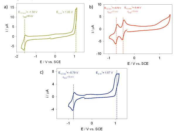
**Figure 6-4** Cyclic voltammograms of a) Y-Per 4-5 (0.51 mM), scan rate 0.05 V/s; b) R-PDI 4-2 (5.0 mM), scan rate 0.05 V/s; c) B-NDI 3-24 (0.64 mM), scan rate 0.03 V/s in DMF at rt with Ferrocene as internal reference;  $E_{Fc+/Fc}$ =0.46 V vs. SCE.
