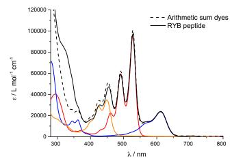
Figure 4-37 Absorption spectra of RYB peptide 4-23 in DMA normalized on B-NDI with arithmetic sum of absorption of dyes B-NDI, R-PDI, Y-Per in DMA.
