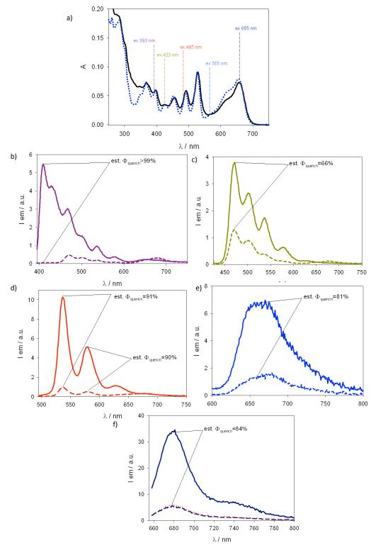
**Figure 6-50** a) Absorption and emission spectra pentad **5-64** and mixture of free dyes (dashed line) used to evaluate the emission quenching on pentad **5-64** (dashed lines): b) Y-Py ( $\lambda_{exc}$ =393 nm), c) Y-Per ( $\lambda_{exc}$ =423 nm), d) R-PDI ( $\lambda_{exc}$ =485 nm), d) B-NDI ( $\lambda_{exc}$ =565 nm), e) B-Cy ( $\lambda_{exc}$ =655 nm).
