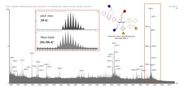
**Figure 5-40** MALDI-Tof analysis of peptide **5-64**; Inset: Zoom of  $[M(-2H)-I]^+$  peak (bottom) compared with calculated mass  $[M-I]^+$  (top).
