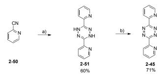
Scheme 6-6 Synthesis of dipyridyl-s-tetrazine 2-45; a) hydrazine hydrate, 90 °C, 12 h; b) DDQ, toluene, 110 °C, 12 h.
