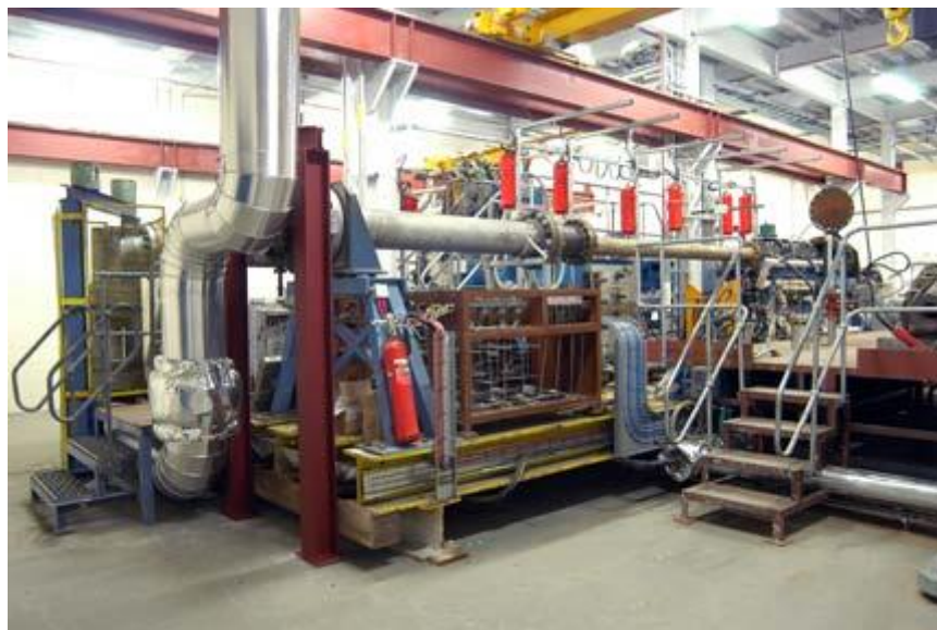
Figure 3-4 Photograph of high pressure combustor rig
