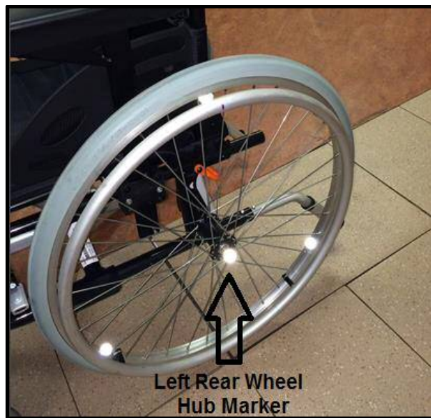
Figure (3.11): Retro-reflective markers placement on the wheel.
