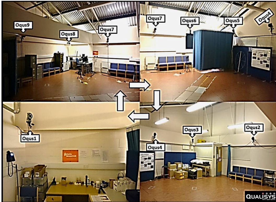
Figure (5.1): Layout of the Motion Analysis Lab at Cardiff University showing Qualisys Pro-Reflex Oqus Cameras arranged around the periphery of the laboratory's walls.
