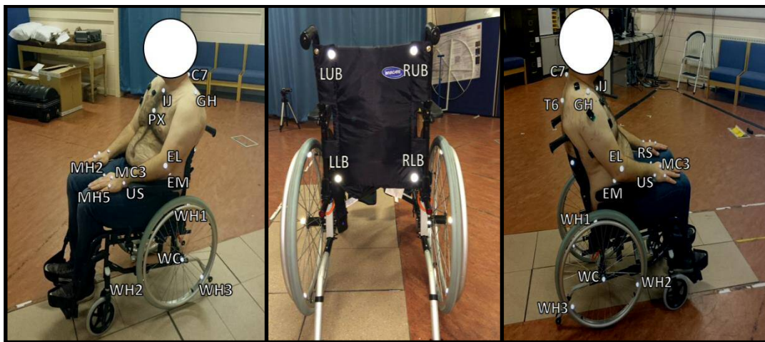
Figure (6.1): Trunk, right and left upper limbs and wheelchair markers set placement.
