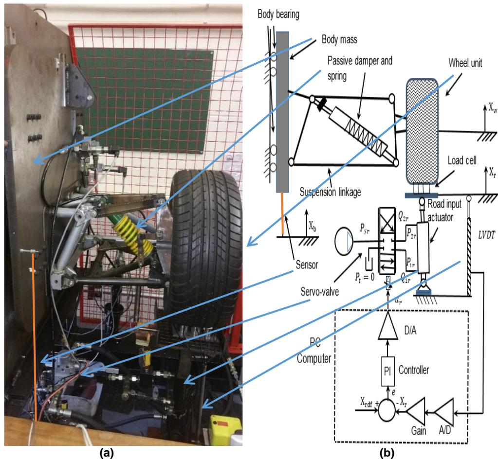
Fig 1 a. Photograph of the test rig b. Schematic diagram of test rig and road simulator
