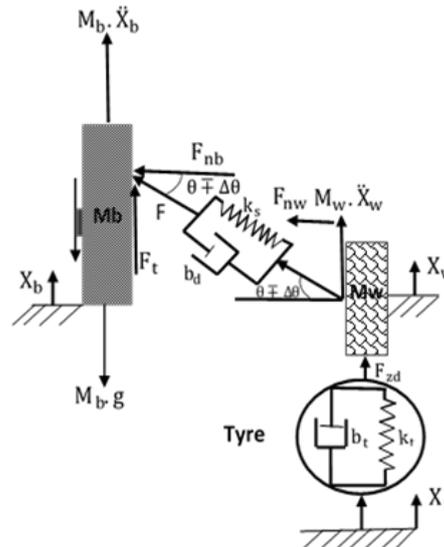
Fig 4 Free body diagram of test rig
