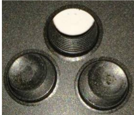
Figure 7.2: Screw holes with tapered geometry and frangible elements
