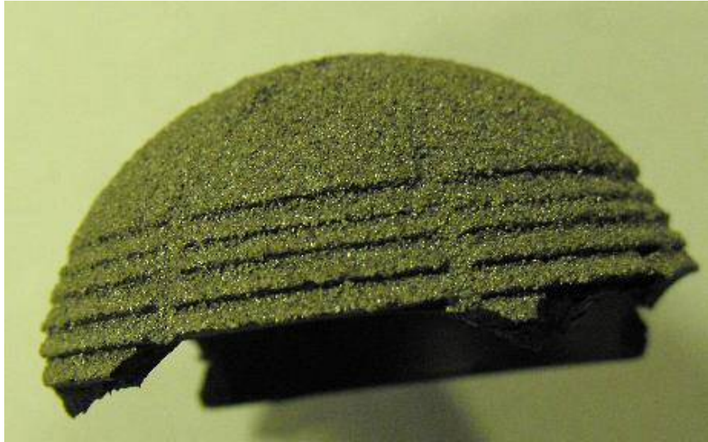
Figure 5.15: Notch sensitivity of PEEK
