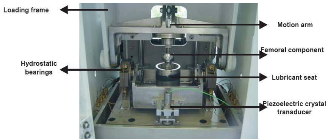
Figure 4.4: The friction measuring carriage and loading frame (Adapted from ProSim (Yan, Neville et al. 2009))
