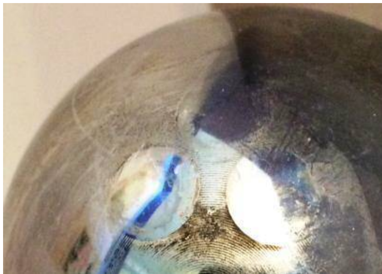
Figure 7.9: Adhesive wear pattern
