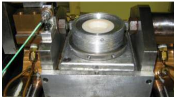
Figure 4.2: Friction testing fixture
