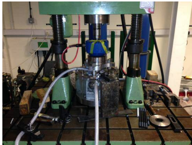
Figure 7.6: Finished fatigue test set-up
