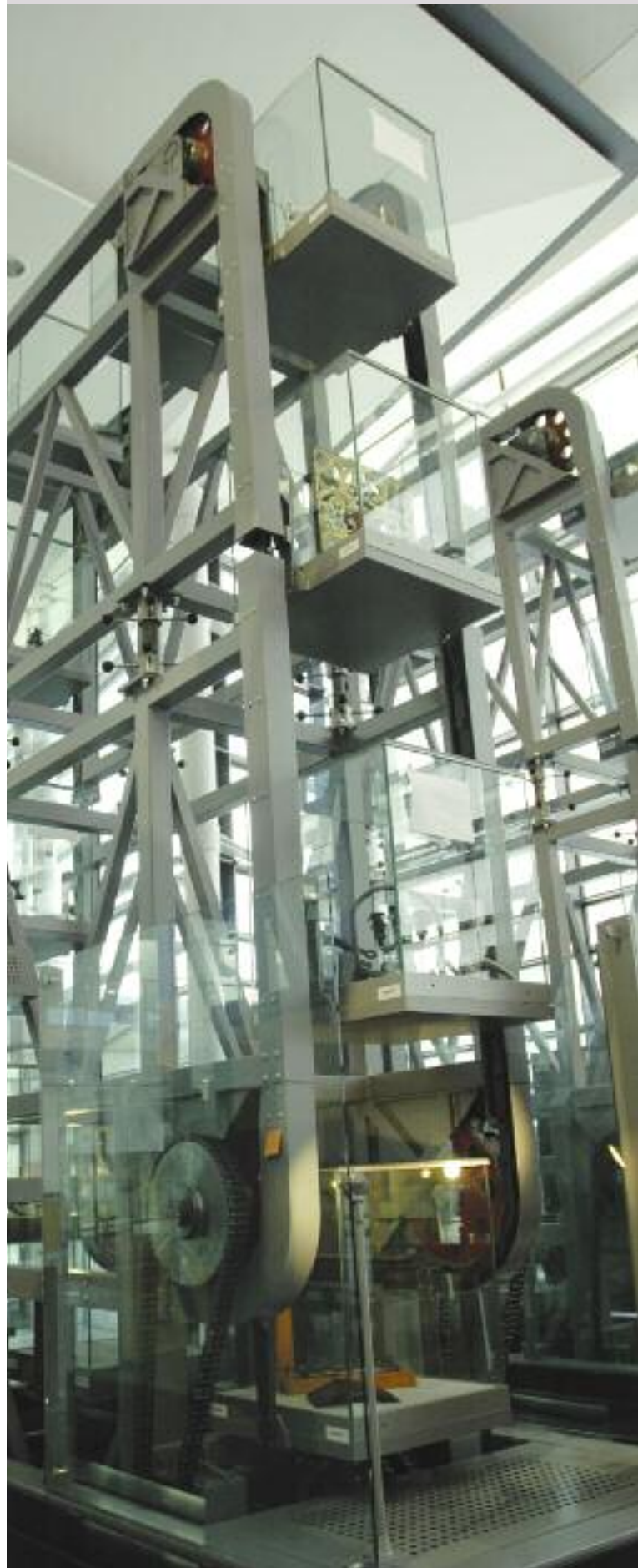
A large revolving paternoster lift which brings objects to the visitors as the cases revolve at the National Waterfront Museum in Swansea
