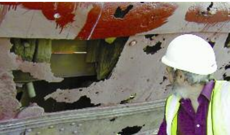
Figure 11. Missing sections of the upper hull
