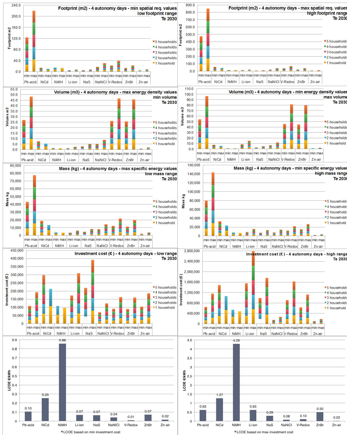
Figure 3. Comparison among footprint, volume, mass, investment cost and LCOE of battery technologies for four days of autonomy in Te 2030
