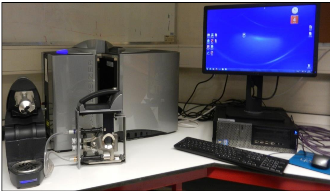
Figure 3.3 Malvern master sizer instrument for measuring particle size distribution
