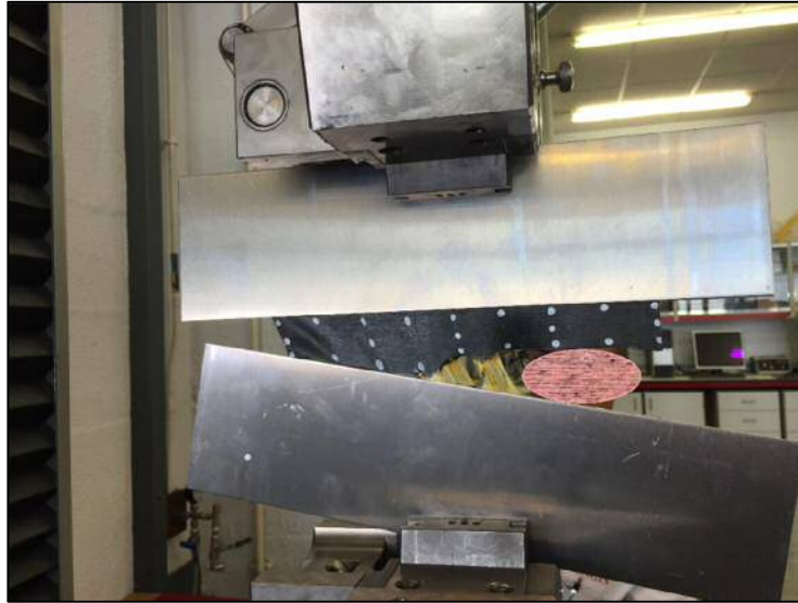
Figure 4-4 Failure of the original clamp design due to slipping of the metal plates and the machine clamps. Instead of tearing of the test piece in the horizontal central line, the material failed from the adhering attachment to the brackets showing no alteration to the painted strain gauges.
