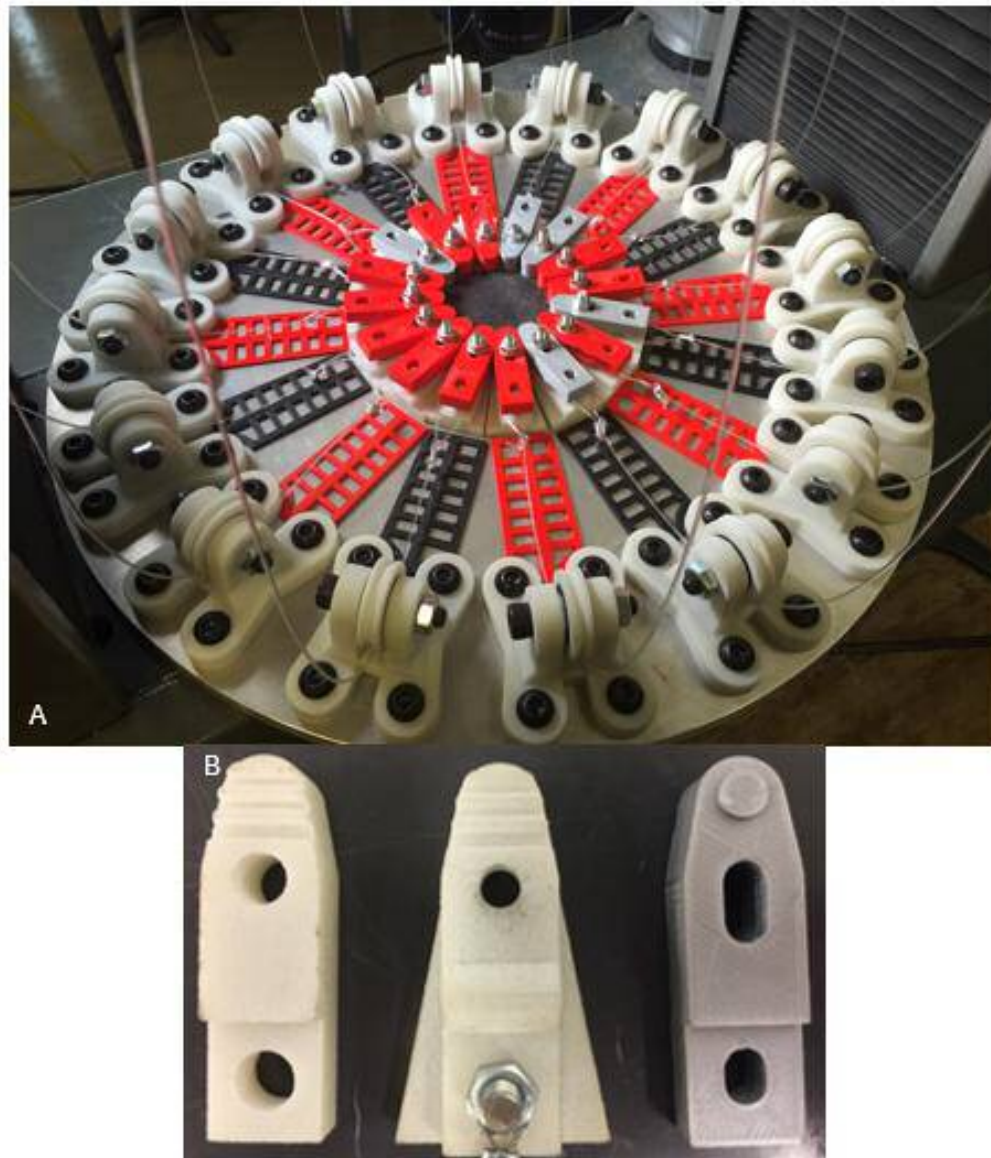
Figure 3-10 (A) Biaxial stretching apparatus with the test specimen in the middle attached to the gripping clamps, (B) The different gripping clamps, the clamp on the left was used instead of the one on the left to accommodate the grooving of the middle lower clamp to avoid stretching the test piece.
