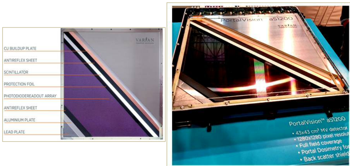
Figure 2.4 - i) A cut out layer of the new Varian PortalVision aS1200 consisting of the detector elements and also a built-in lead plate as shielding from the linac arm backscatter.
