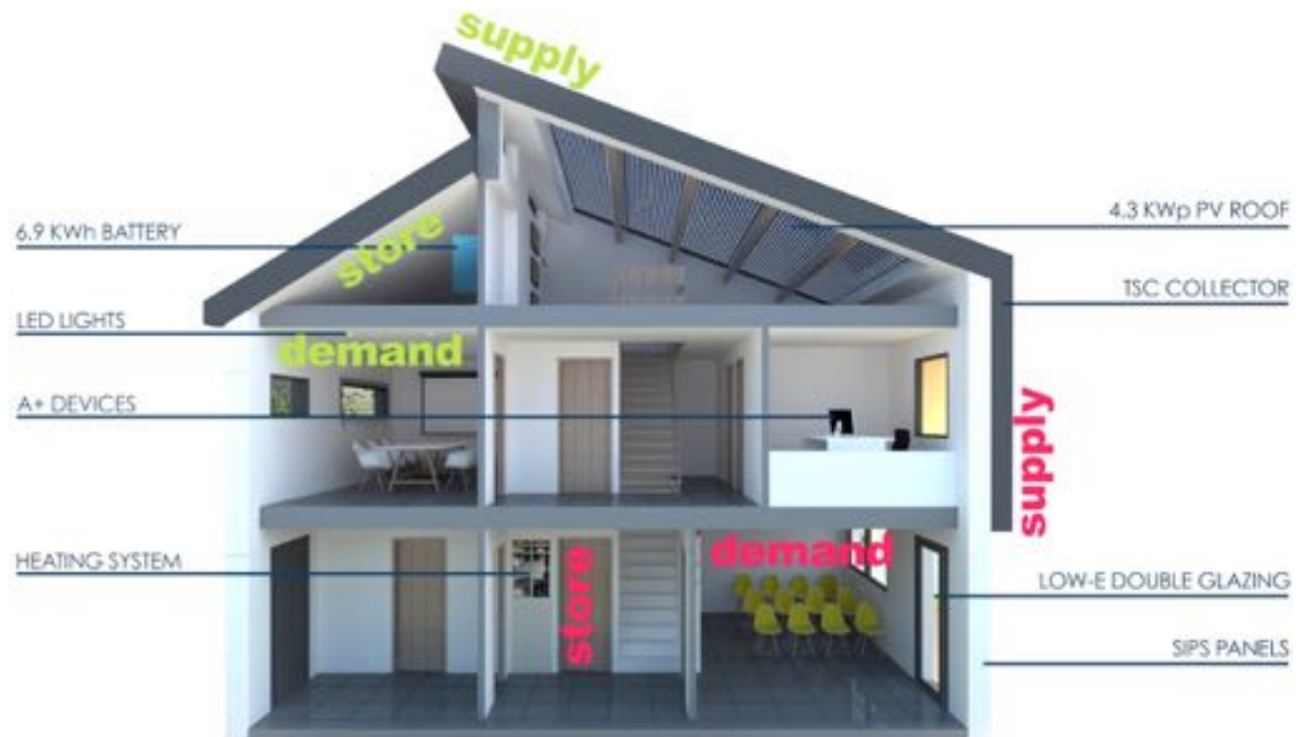
Figure 123 – Schematic of the EPH design showing the novel technologies and construction methods used.
