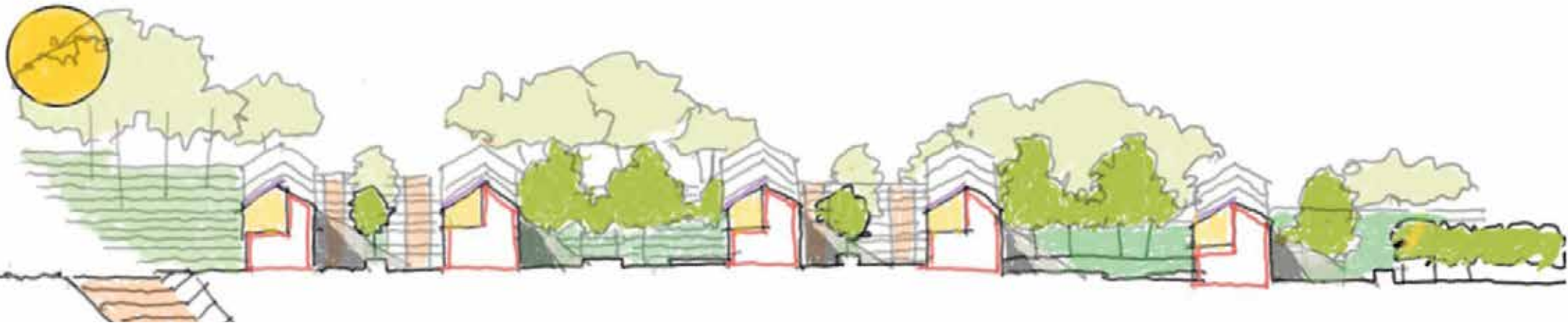
Fig 21: Solar Path and Building Orientation
