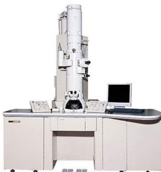
Figure 47. JEOL JEM 2100 Electron Microscope.
