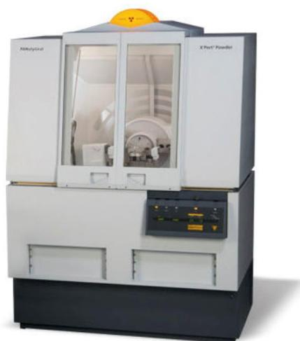
Figure 42. PANalytical X'PertPRO X-ray diffractometer.
