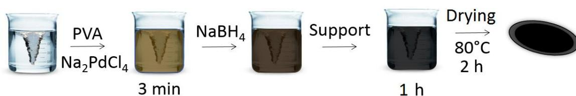
Scheme 2. Schematic representation of the sol-immobilisation process used in this Thesis.
