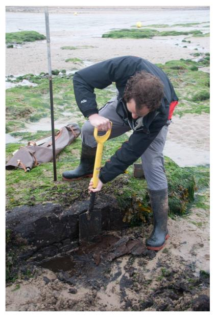
Figure 42: Cutting a vertical section through intertidal deposits at Port Eynon
