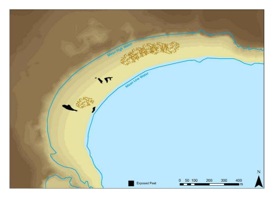
Figure 50: Locations of peat exposures at Port Eynon following the GPS survey
