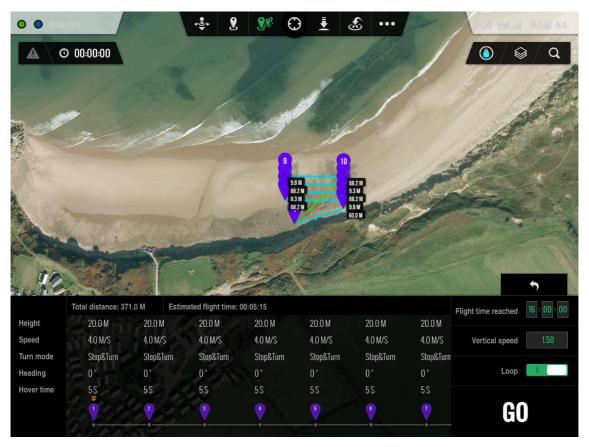
Figure 28: Flight plan for drone survey of upper beach peat exposure at Broughton Bay created using the DGI Ground Station app
