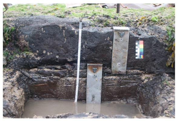
Figure 44: Overlapping monolith tin placement
