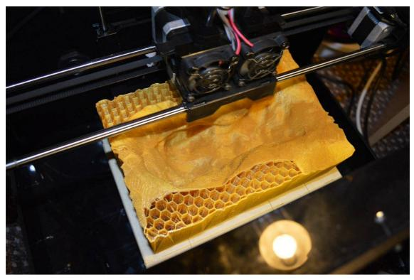
Figure 41: Overhead shot of footprint being printed. The inside of the model was designed to be honeycomb in structure to reduce the amount of material needed, while maintaining the object's strength (Paul Smith 2015)
