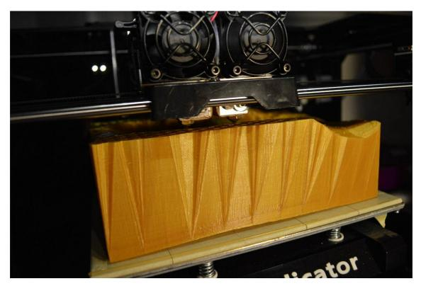
Figure 40: Side view of footprint being printed on a MakerBot Replicator 3D printer (Paul Smith 2015)
