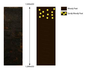
Figure 71: Sediment column sample Br4
