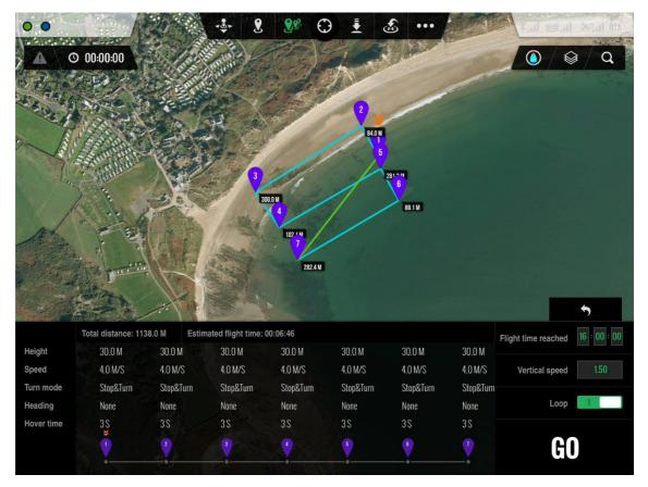
Figure 30: Flight plan for survey of Port Eynon peat exposure in the lower intertidal zone created using the DGI Ground Station app
