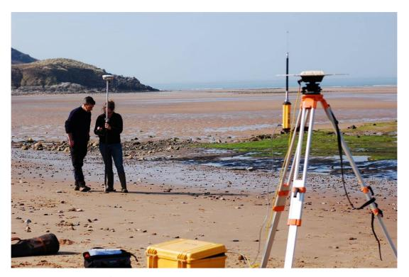
Figure 23: Trimble 4700 base station and Trimble 5800 Rover in use at Broughton Bay
