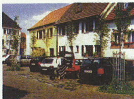
The roadway is one way (3 metres wide), but could be two way without compromising the design idea. Trees are given adequate protection against manoeuvring cars and vandalism
