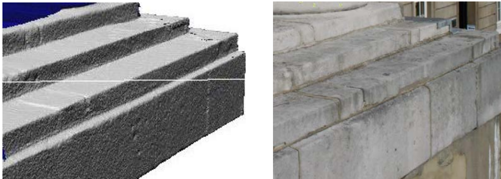
Figure 4 – Comparison of part of a historic building using laser scanning (left) and the image taken from a similar viewport in reality (right).
