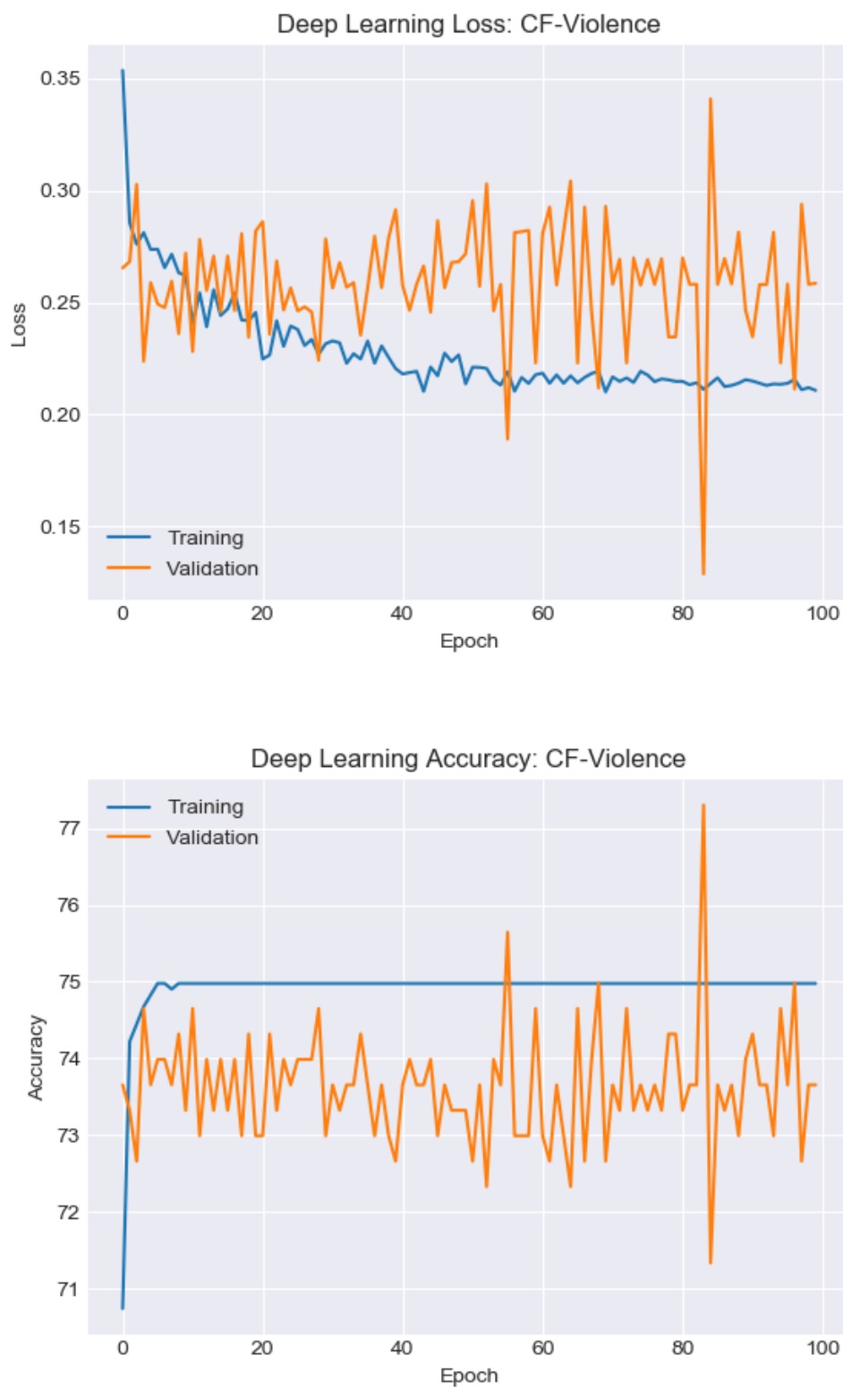
Figure 5.11: Training and validation accuracy/loss when fitting a C3D model using the CF-Violence dataset.
