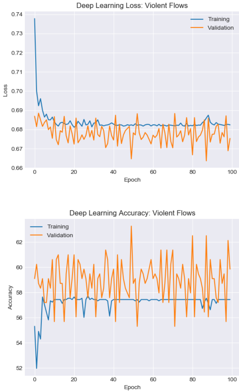
Figure 5.14: Training and validation accuracy/loss when fitting a C3D model using the Violent Flows dataset.
