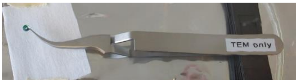
Figure 2.2 A photo shot showing the NP settlement step: a steel reverse action tweezers was lying flat in a glass container, the tip of the tweezers held the frame of the sample grid with 9 \mu\text{L} NP solution covering the top surface of the grid.
