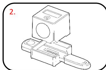
Replace cap. The pink liquid will start to migrate up the test strip. The green line will be replaced with a red line – the control line. Insert into the adaptor and place the cube reader on top
