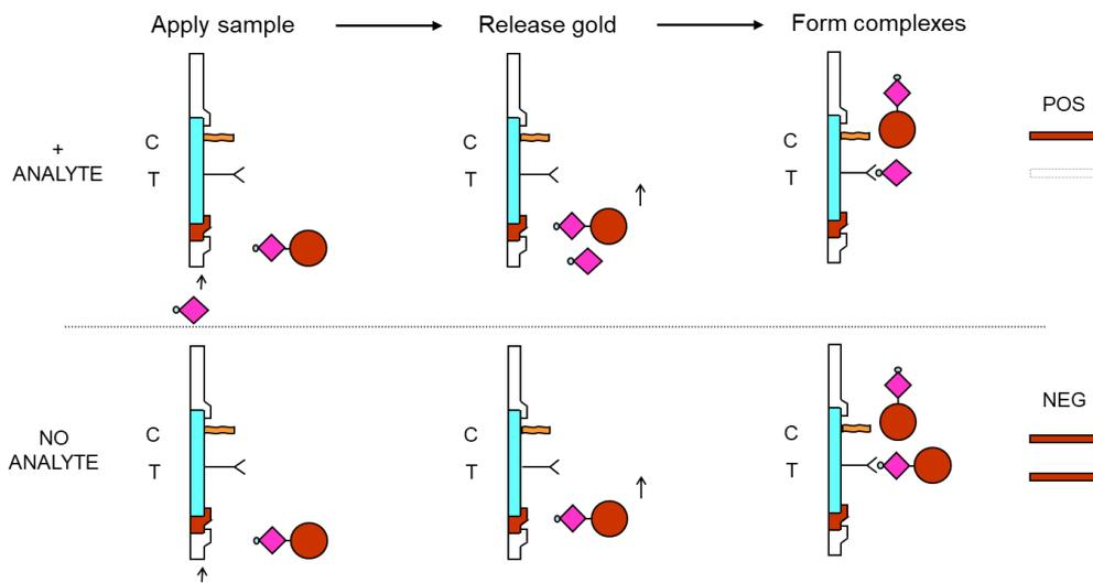
Figure 5.3. A competitive assay format. The analyte in the sample competes with the analyte-detector conjugate i.e. gold with the antibody immobilised on the nitrocellulose membrane. With unlabelled analyte bound to the antibody test line, there is an absence of a visible line.
