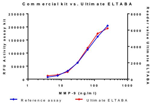
Figure O. Comparison of Ultimate ELTABA with commercial kits. A graph comparing the ability of a commercially available active MMP assay kit and Ultimate ELTABA with the same standard applied to both assays.
