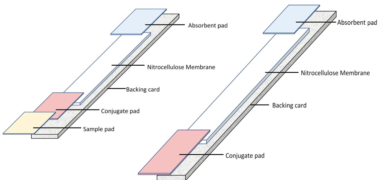
Figure 5.8. Visual representation of the different strip architecture. Version 1 being a shorter strip and with a sample pad and version 2, a longer strip with a wick added during assembly.
