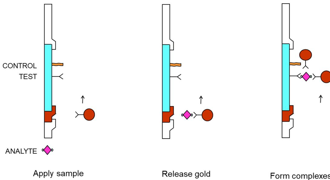
Figure 5.2. A sandwich assay format. The analyte in the sample forms a complex with the primary antibody-detector conjugate i.e. gold which then forms a complex with a secondary antibody immobilised on the nitrocellulose membrane forming a visible line. A control line in this example is an anti-species to the primary antibody.
