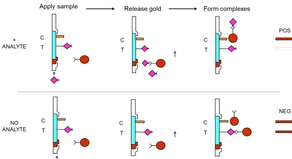
Figure 5.4. An inhibition assay format. The analyte in the sample inhibits binding of the detector reagent at the test line by forming a complex with the antibody-detector conjugate i.e. gold preventing it from binding to the analyte immobilised on the nitrocellulose membrane. With no antibody-detector conjugate bound to the test line, there is an absence of a visible line.
