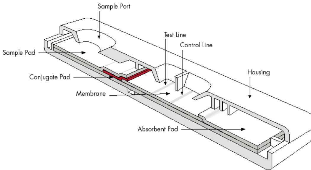
Figure 5.1. A typical lateral flow assay. A strip is enclosed in a plastic housing with a sample port for sample addition and a read window where the result can be interpreted by the user in the form of test lines and control lines (courtesy of Millipore)
