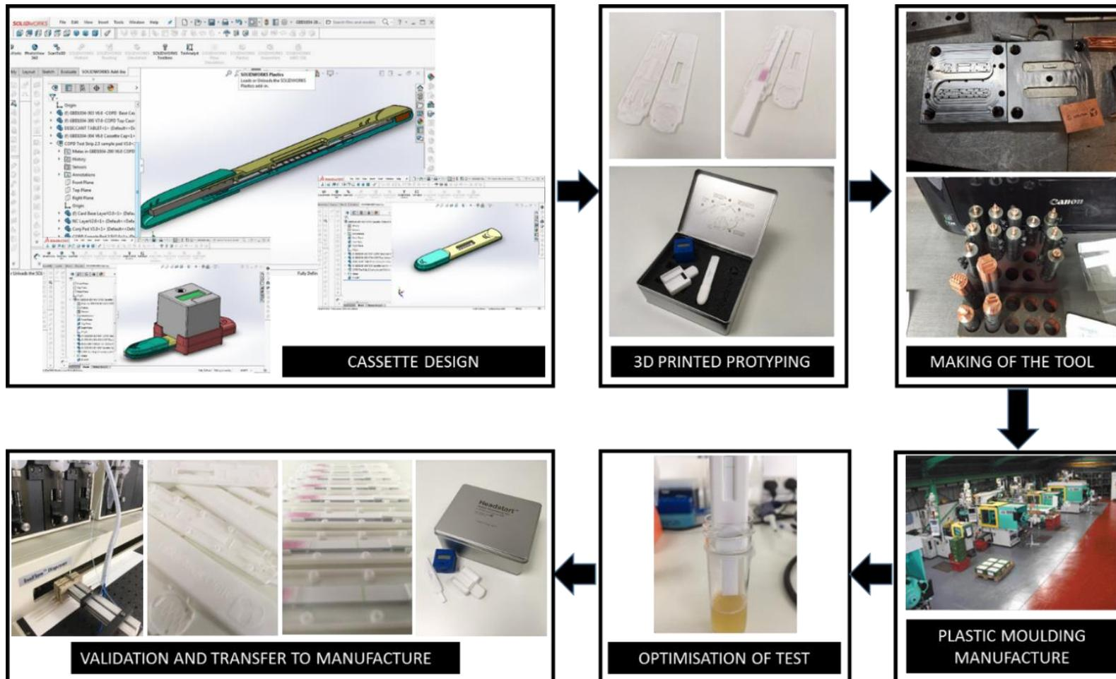
Figure 5.7. Development of plastic housing from point of concept to manufacturing. 3D printed devices were evaluated before committing to the tool development. Which required further refinements before freezing the design and transfer to manufacture.
