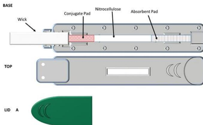
Figure 5.9. Diagrammatic representation of assembly process for test device version 2 with a green lid for A and an orange lid for B. Manual addition of strip and wick but machine closed to ensure equal distribution of pressure.
