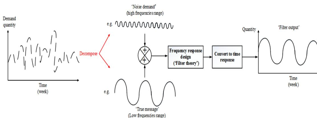
Figure 3. 4. Transmission by the frequency response design
