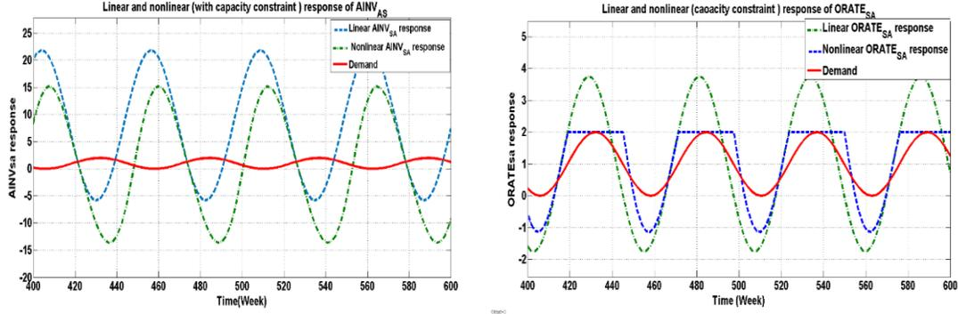
Figure 5. 12. The impact of PC parts supplier capacity constraint (Capacity limit =2) on  $ORATE_{SA}$  and  $AINV_{SA}$ . Note: different scales in the y-axis and control parameter settings:  $\tau_A = \tau_{WIP} = 2\tau_{SA} =$
