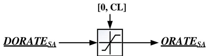
Figure 5. 5. The open loop form of saturation nonlinearity function in the supplier system extracted from Figure 5.3.
