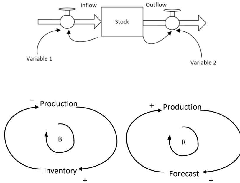
Figure 3. 8. The introduction of the stock-flow diagram and balancing and reinforcing casual loops
