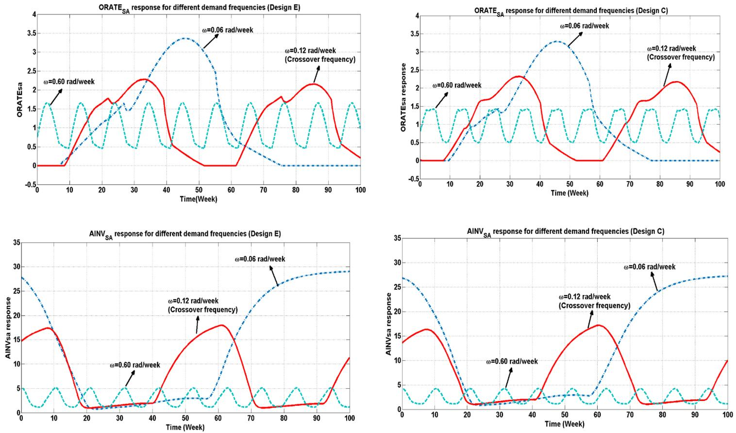
Figure 5. 7. Delivery LT,  $ORATE_{SA}$  and  $AINV_{SA}$  response for sinusoidal demand (Mean=Amplitude=1) with different frequencies ( $\omega=0.06$  rad/week,  $0.12$  rad/week and  $0.60$  rad/week) in the nonlinear ATO system
