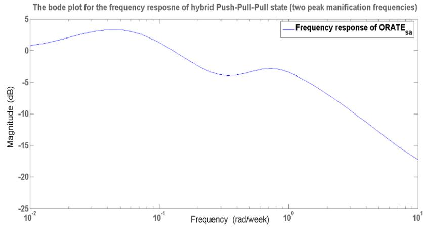
Figure 5. 4. An example of the frequency response of  $ORATE_{SA}$  for the *Push-Pull-Pull* state with two peak magnification frequencies ( $\tau_A = 16$ ,  $\tau_{AINV} = \tau_{WIP} = 24$ ,  $\tau_{SA} = 8$ ,  $\tau_{DD} = 0.5$ ,  $\tau_I = 2$ ,  $\tau_{AS} = 1$ )
