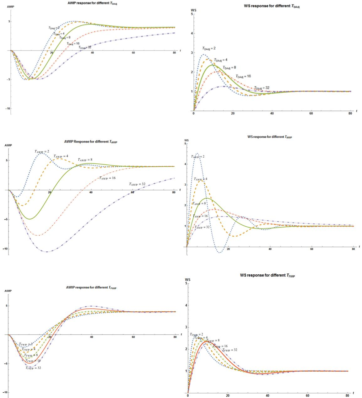
Figure 4. 7. The effect of decision policies for the AWIP and WS in response to unit step increases.
