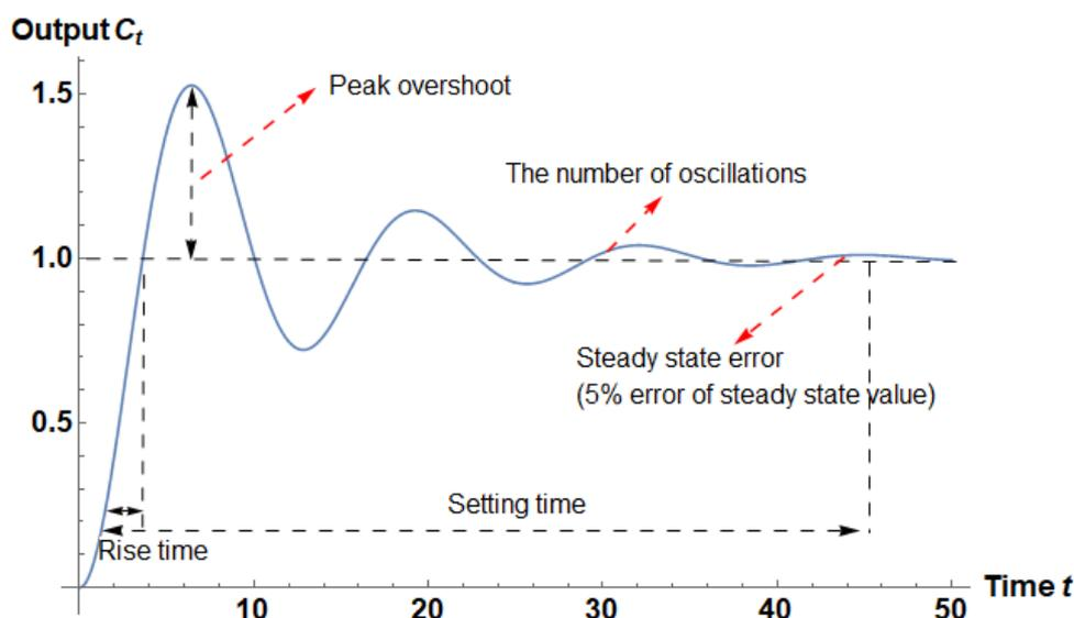
Figure 3. 5. Performance evaluation of time domain analysis via the ‘shock’ lens (i.e. a unit step demand increase).
