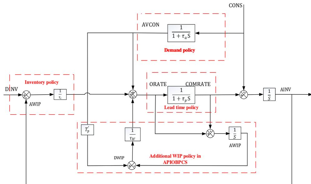
Figure 3. 11. Block diagram representation of APIOBPCS (including IOBPCS) archetype.
