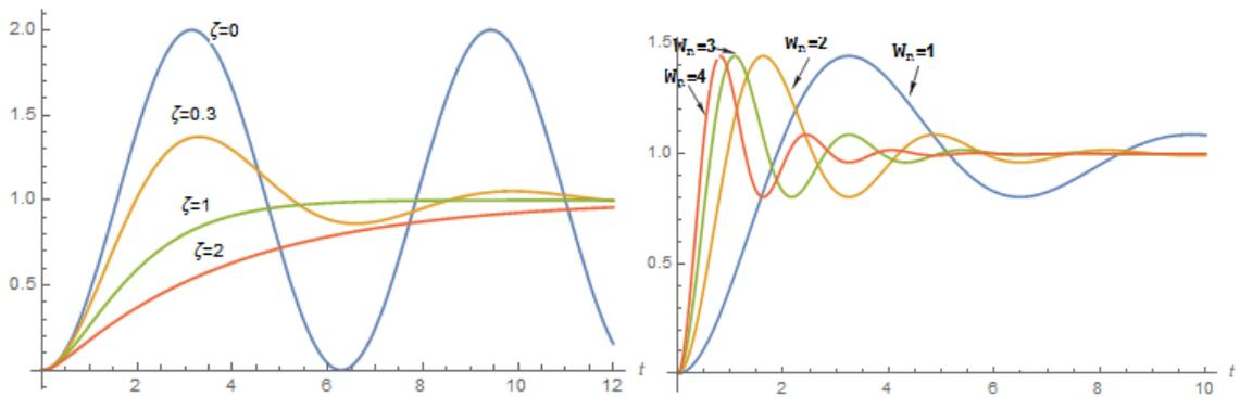
Figure 3. 7. Examples for the effect of  $\omega_n$  and  $\zeta$  in responding to a unit step input.
