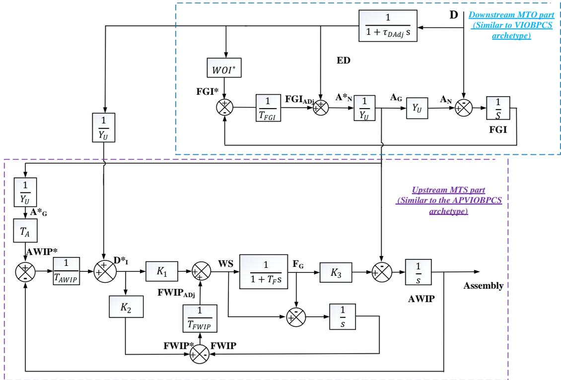
Figure 4. 4. Re-arranged block diagram for the hybrid ATO supply chain model.
