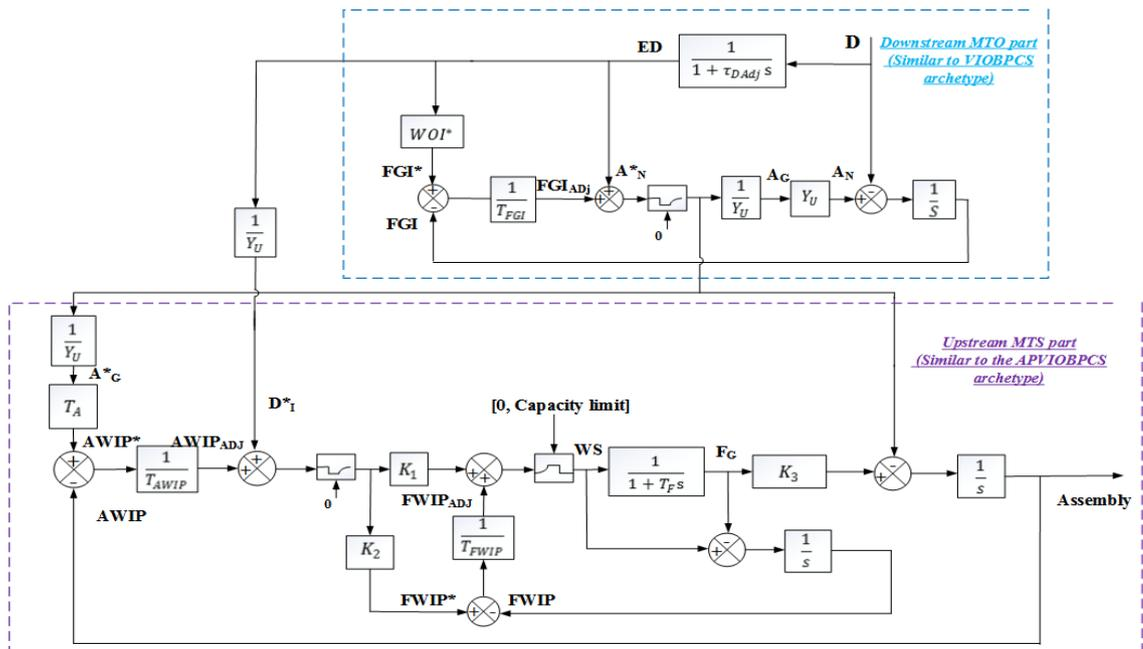
Figure 4. 9. The semiconductor hybrid ATO supply chain in the nonlinear block diagram form.
