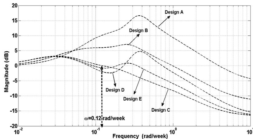
Figure 5. 6. Five basic designs for  $ORATE_{SA}$  response under Push-Pull-Pull state
