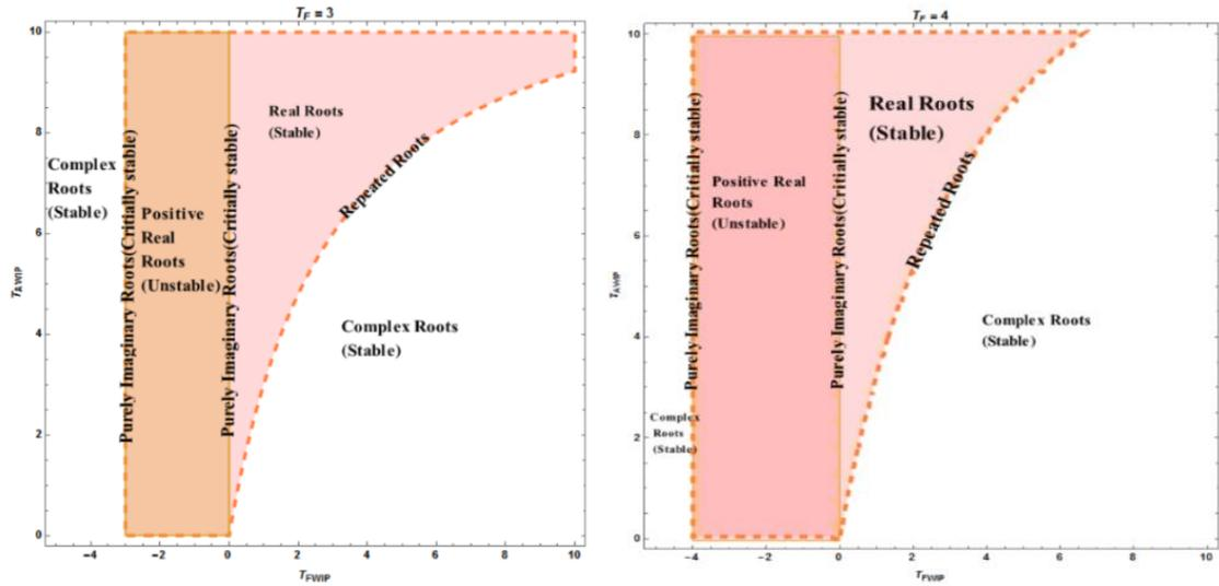
Figure 4. 6. Real, complex and imaginary region of  $R_3$  and  $R_4$  based on different  $T_F$ .
