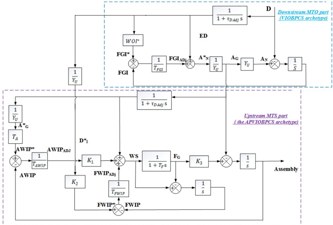
Figure 4. 8. The APVIOBPCS-based hybrid ATO in block diagram form
