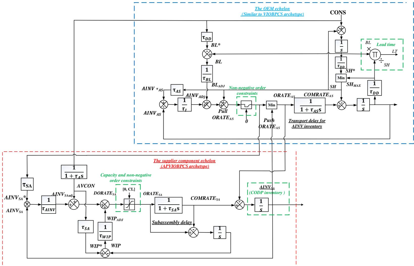
Figure 5. 2. System dynamics model for the PC hybrid ATO supply chain.
