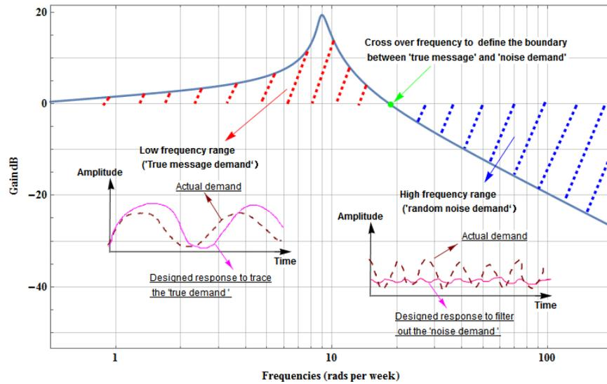
Figure 3. 6. Frequency response illustrated by Bode plot diagram. Adapted from Towill (1994) and Towill et al. (2003).
