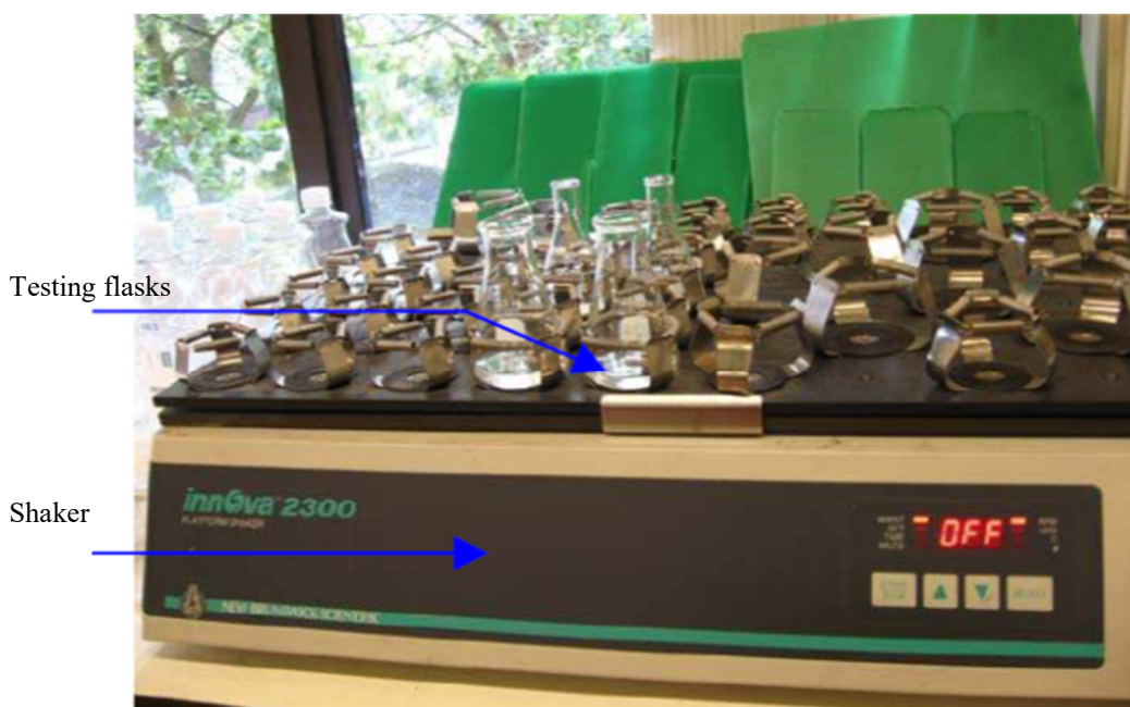
Figure 3.18 Reciprocal shaker and sample flasks
