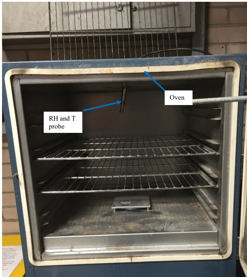
Figure 3.11 Photograph showing the calibration of the temperature probe
