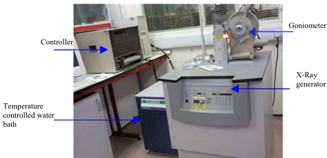
Figure 3.1 Philips automated diffractometer PW1710 used in this study
