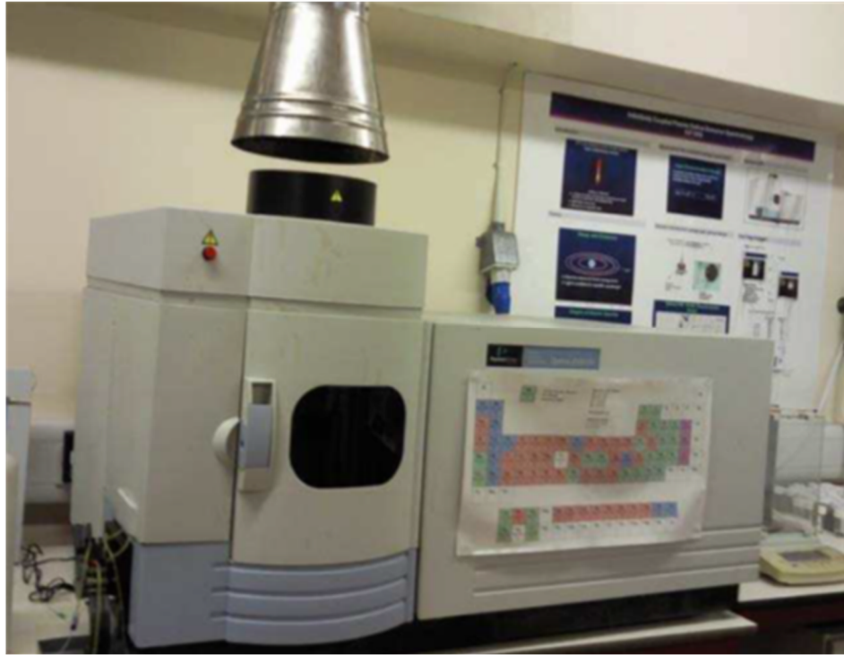
Figure 3.19 Perkin Elmer Optima-2100 DV Inductively Coupled Plasma Optical Emission Spectroscopy (ICP-OES)
