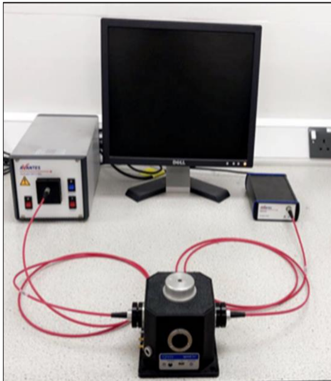
Figure 2.4 photograph of the AvaSoft UV-Vis Spectrometry setup (On-line batch reactor) for monitoring the reduction of 4-nitrophenol. (Cardiff Catalysis Institute).
